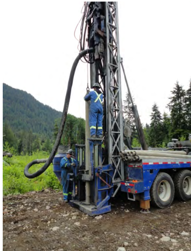
Figure 10. A Becker hammer drill at McNab Creek. Photo courtesy BURNCO Rock Products Ltd.
