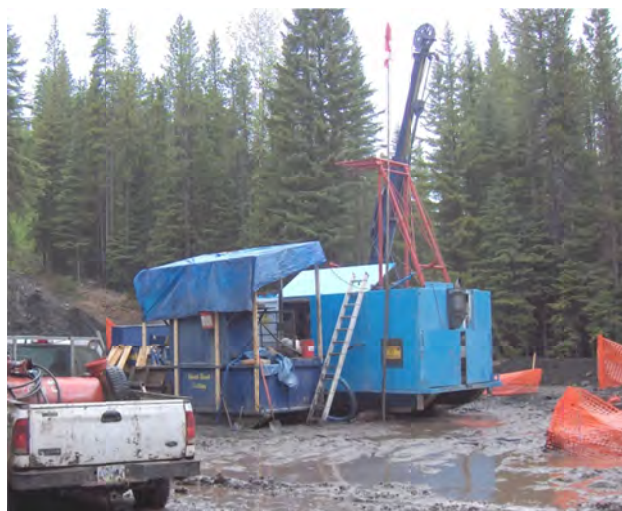
Figure 18. Diamond drilling on the Bingay Creek coal property
