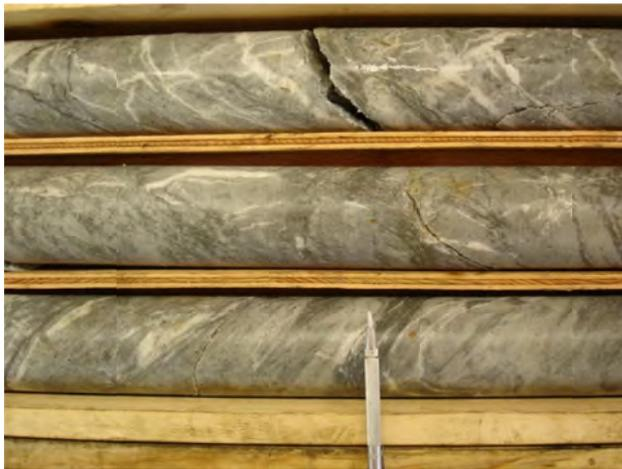
Figure 36. Brucejack project; Shore zone SU-105, foliated quartz-sericite-pyrite alteration, protolith unknown.
