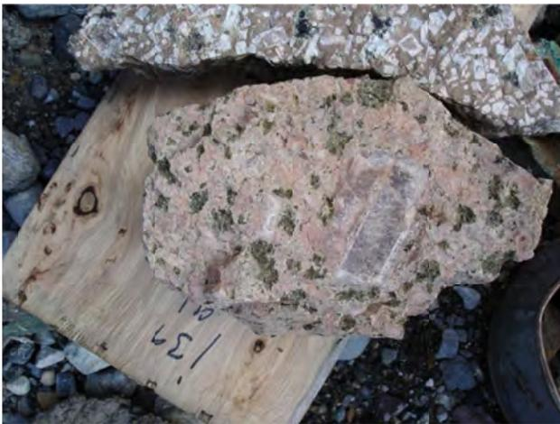
Figure 50. Dirk zone southeast of Trek; K-feldspar porphyry syenite (with epidote) and pseudoleucite porphyry are associated with copper mineralization.
