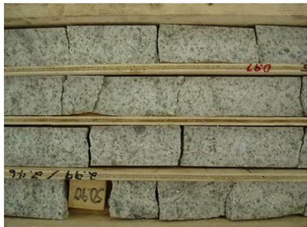
Figure 62. Lone Pine; quartz porphyry in the Alaskite and 66 molybdenum zones.
