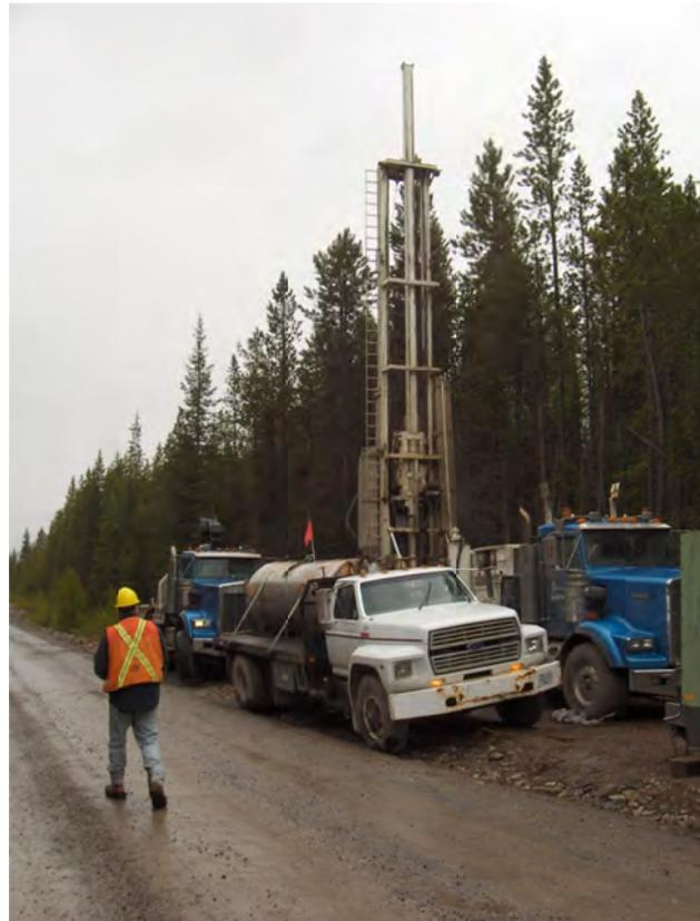
Figure 17. Rotary drilling at the side of the Elk Valley Forest Service Road north of Elkford on Centremount Coal Ltd's Bingay Creek coal property.
