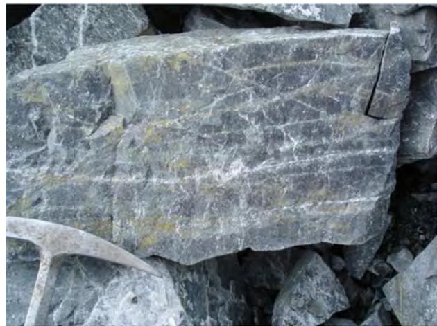
Figure 7. Huckleberry copper mine; ore from the MZX pit, biotite hornfels with chalcopyrite and gypsum filling fractures.
