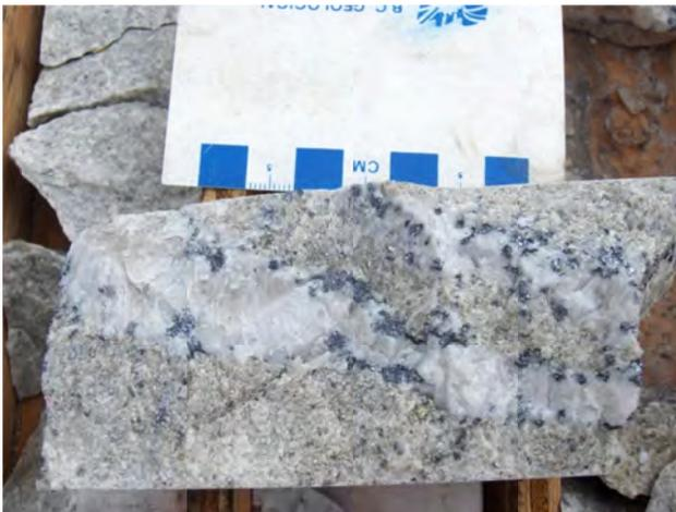
Figure 6. Molybdenite-bearing quartz veining from the Ethyl zone at the MAX molybdenum mine.
