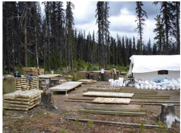
Figure 24. Capoose, core logging, sampling and storage facility within pine beetle-killed forest.
