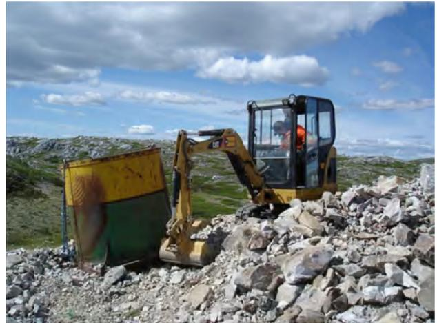
Figure 33. Nonda bulk sample rock being loaded into helicopter bucket.
