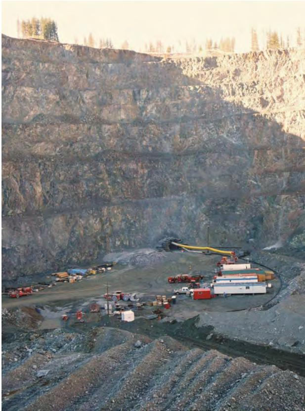
Figure 18. The bottom of the Wight pit at the Mount Polley copper-gold mine was used to start a decline to facilitate testing the Boundary and Zuke zones where the potential for underground mining is being considered.
