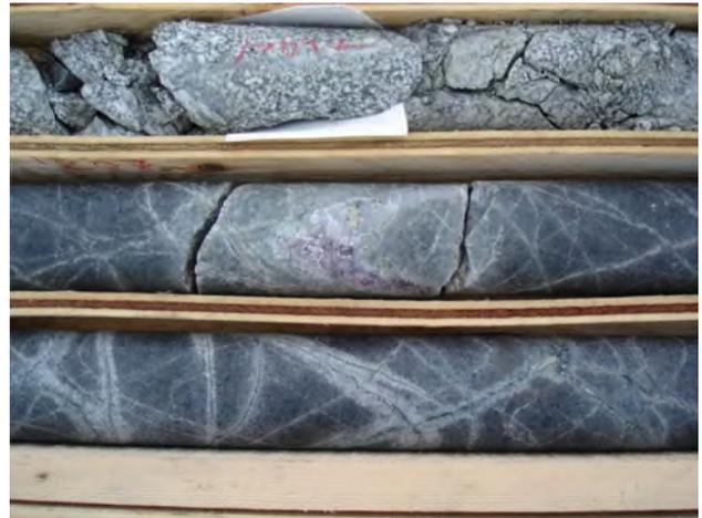
Figure 53. High Gold project; fracture-veined hornfels and granodiorite, containing quartz, sulphides and purple anhydrite.
