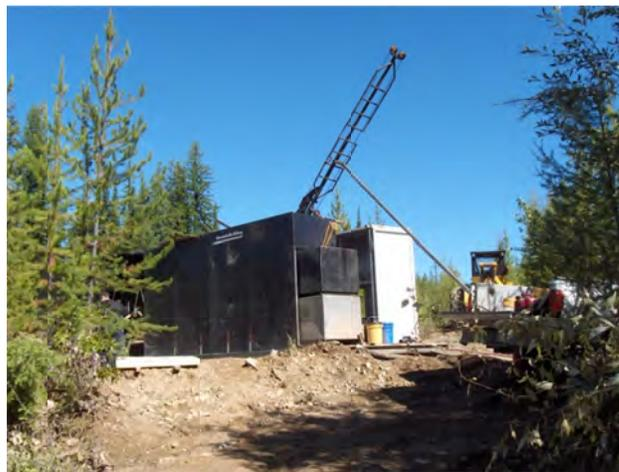
Figure 10. Diamond drilling on Astral Mining Corporation and Kootenay Gold Inc's Jumping Josephine property.
