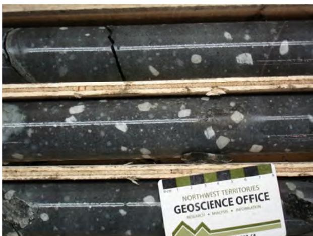
Figure 65. Lone Pine molybdenum project; intramineral K-feldspar porphyry.
