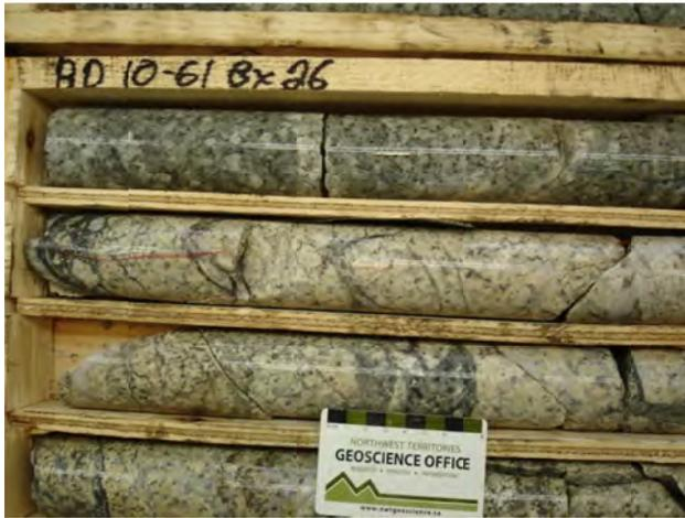
Figure 63. Lone Pine; fractured granite porphyry and quartz-molybdenite veins in the 66 zone.
