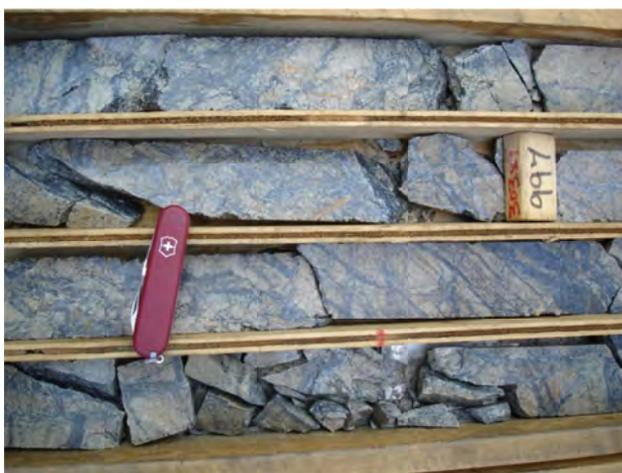
Figure 10. Kwanika Central zone, supergene chalcocite in quartz stockwork with overprint of albite-Fe-carbonate-hematite alteration, from drillhole 62.
