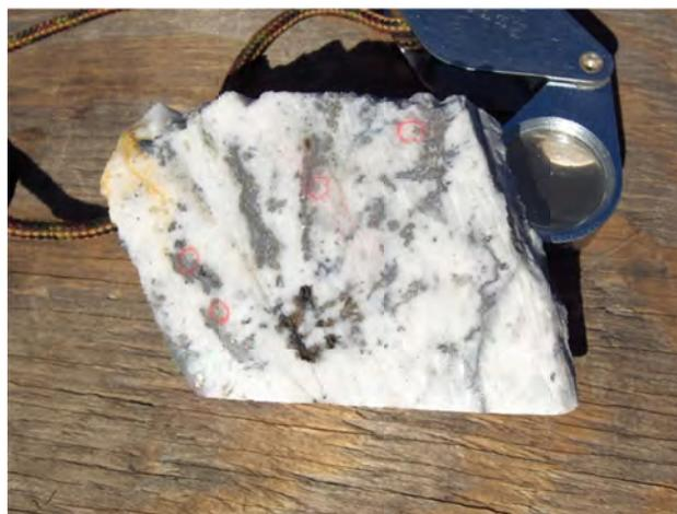
Figure 11. Pyrite, arsenopyrite and gold (inside red circles) in quartz vein material, Jumping Josephine property drill core.
