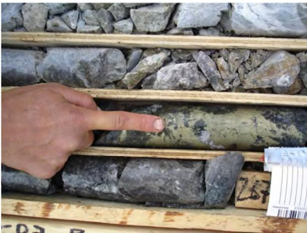
Figure 49. Trek project; chalcopyrite vein in mafic volcanic rock.
