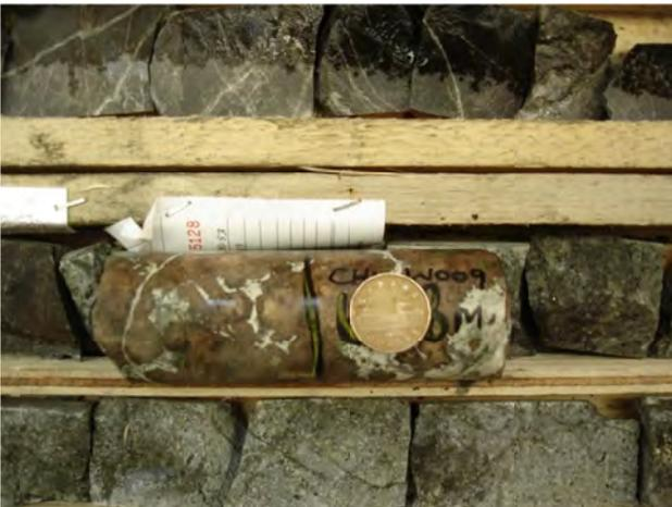
Figure 8. Chu, hydrothermal spessartine garnet in drill core; also visible are fractured siltstone hornfels and granodiorite.
