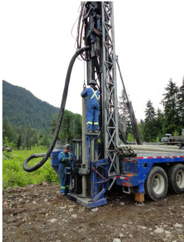
Figure 10. A Becker hammer drill at McNab Creek. Photo courtesy BURNCO Rock Products Ltd.
