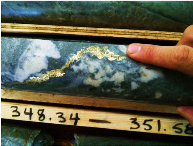
Figure 14. Gold vein in drill core from Brucejack. Twenty-four intercepts drilling in 2011 graded over 1000 g/t Au. Photo courtesy of Cole Mooney.
