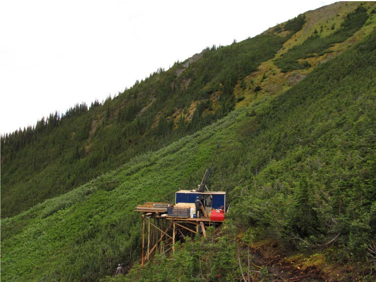
Figure 7. Diamond drilling on the Northwest extension of the Akie SEDEX project (courtesy Canada Zinc Metals).
