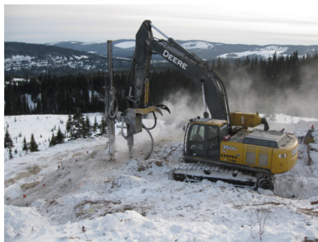
Figure 9. Drilling blast holes for bulk sample at the Angus property (courtesy Stikine Energy).
