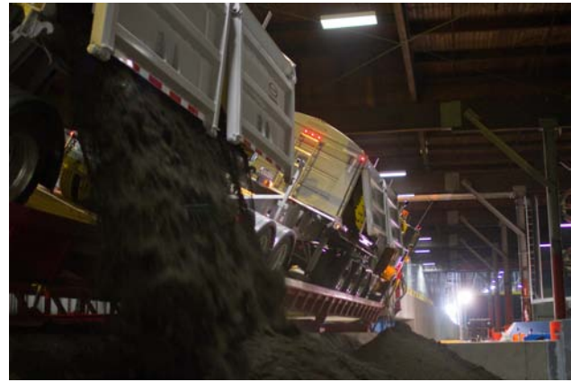
Figure 4. Ore concentrate load out facility for the Copper Mountain mine where the first concentrate was shipped (courtesy of Copper Mountain Mining Corporation).
