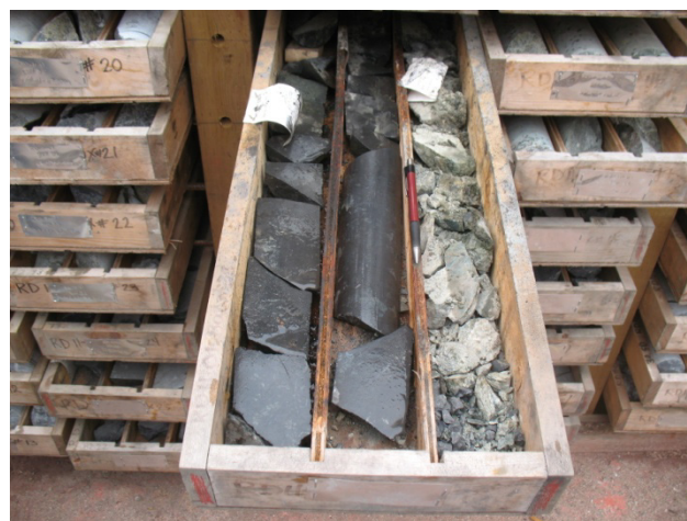
Figure 13. Massive magnetite at the Brynnor project. Brynnor is a 1960s past-producer of iron ore, one of several magnetite skarns on the coast that are subject to re-examination in light of recent demand for iron ore.
