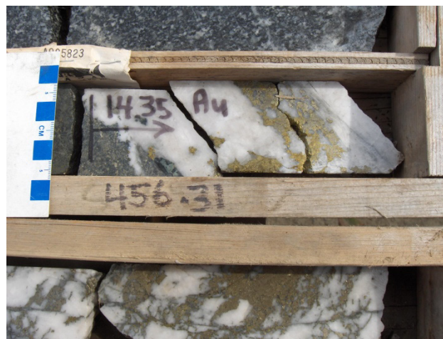
Figure 10. Recent drill-core from the Kenville Gold Mine Project (Anglo Swiss Resources Inc). High-grade gold in the core is associated with pyrite and chalcopyrite in a quartz vein. "Pseudodiorite" of the Eagle Creek pluton is also visible.
