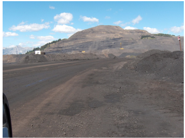
Figure 7. Elkview Operations of Teck Coal Limited. The BR-1 Pit high-wall at the south end of Baldy Ridge is visible in the distance. The new BR2 expansion area, approved in late 2011, will be north of BR1.
