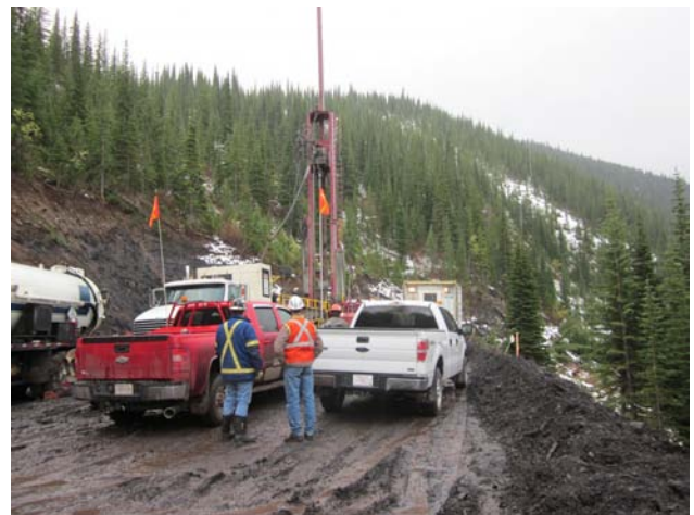
Figure 17. Rotary drilling on the Marten-Wheeler Project (Teck Coal Limited).
