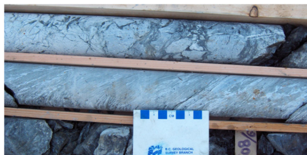
Figure 12. Recent drill-core from the Talon zone on the Iron Range property (Providence Resources Corp). Albite alteration and breccia textures suggest the possible existence of a hydrothermal vent at Sullivan time in the Aldridge Formation.
