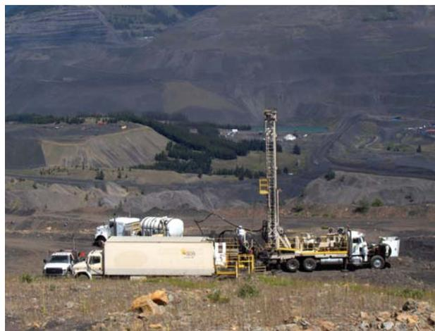
Figure 15. Rotary drilling on the Swift Project, Fording River Operations (Teck Coal Limited).
