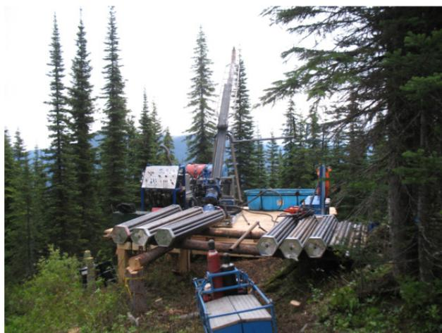
Figure 8. Drill on-site at the Carbo REE project (courtesy Canadian International Minerals).
