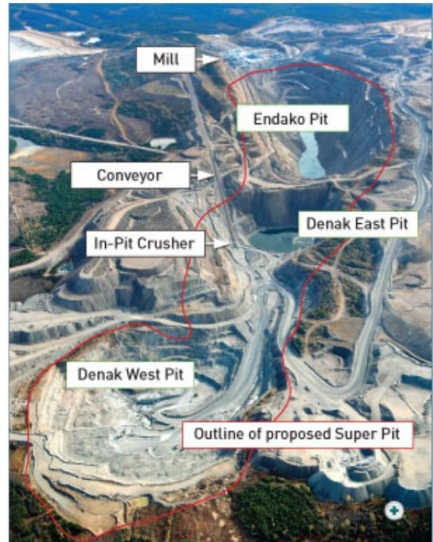
Figure 4. Areal view of Endako Mine showing the 3 existing pits. Courtesy of Endako Mines.
