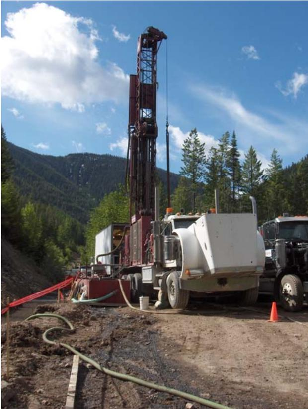
Figure 18. Rotary drilling on the Coal Creek Project (Crowsnest Pass Coal Mining Ltd).
