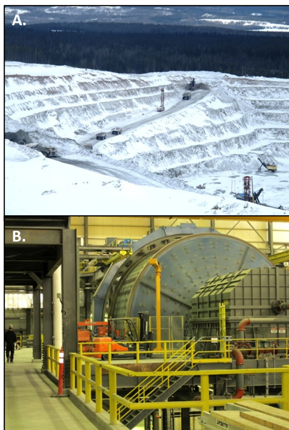
Figure 1.5. Endako Mine – A. Mining in West Denak pit to supply low-grade stockpile; B. New Semi-Autogenous Grinding (SAG) mill.
