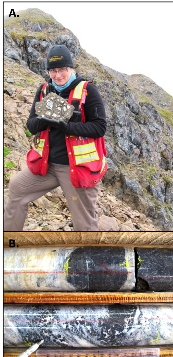
Figure 1.17. Aley project – A. Taseko Mines geologist Mercedes Rich at the carbonatite contact in the Saddle zone with syenite-bearing fenite breccia; B. Niobium ore in dolomitized carbonatite.
