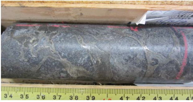
Figure 2.34. Drill hole THN 12-84: high grade polymetallic mineralization.
