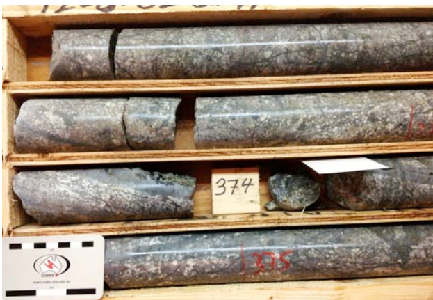
Figure 2.27. Drill hole 12S-02; Itsit feldspar-porphyry with moderate to strong quartz stockwork similar in texture to gold-copper bearing core drilled in 2011.
