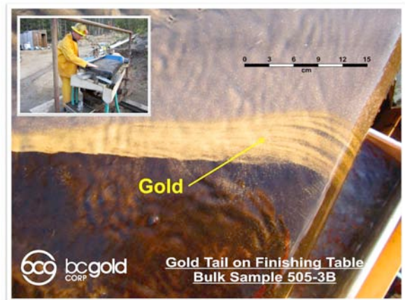
Figure 2.33. The gold line off the wash table at BC Gold Corp's Engineer gold mine. Courtesy of BC Gold Corp.
