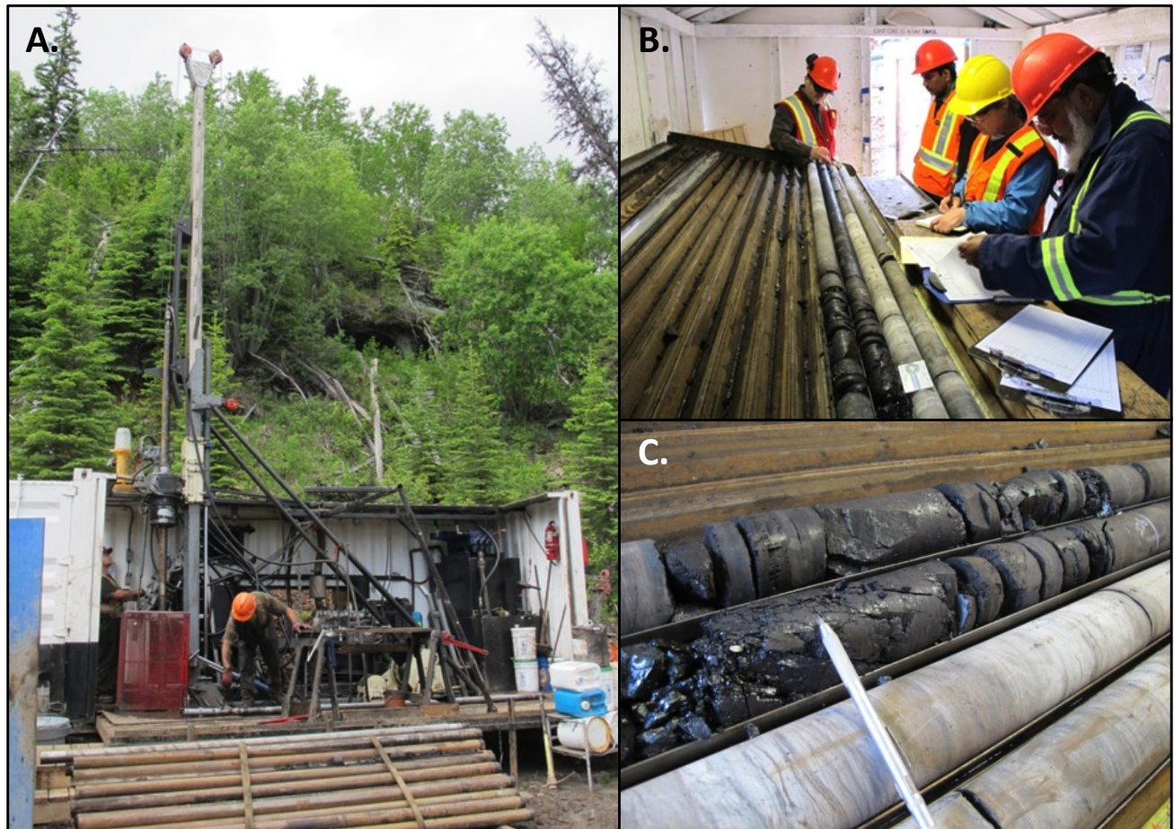
Figure 3.12. Carbon Creek – A. Orofino Drilling Ltd drill using HQ3 system; B. Cardero geologists in core shed reviewing drill logs with Janet Riddell; C. Gething Formation coal seam no. 31 in core.
