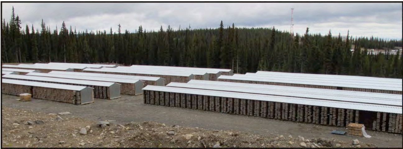
Figure 11. Blackwater – On-site core storage facility for the 2012 drilling program of 700 holes and over 245 000 m of core.
