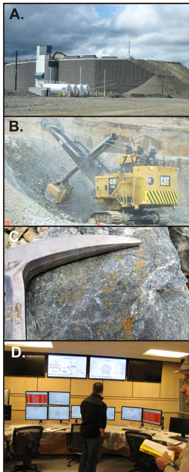
Figure 8. Mt. Milligan Mine – A. Gabion wall of above-ground gyratory crusher tower; B. Phase 1 mining in MBX zone, 7495 electric shovel; C. Copper-gold ore near the brecciated monzonite/andesite contact in the MBX zone; D. Mine dispatch and mill centralized control area.
