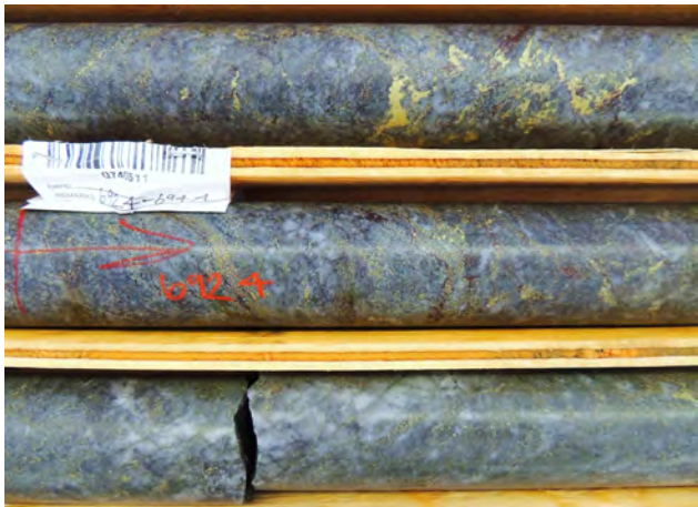
Figure 5. Drilling at Deep Kerr successfully followed up a high-grade copper gold core zone. Hole K-13-29 692.4 m showing very strong pervasive silica replacement with abundant interstitial chalcopyrite and bornite. Photo Credit Mike Savell, Seabridge Gold.
