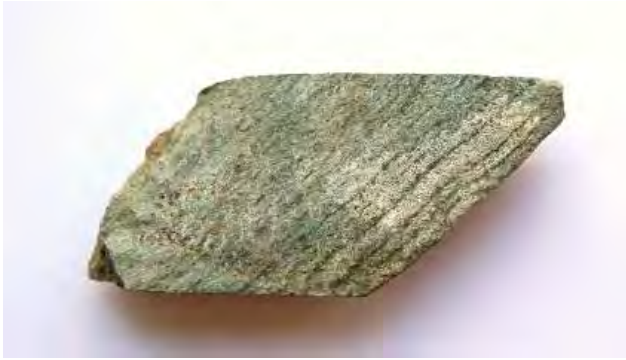
Figure 26. Volcanogenic sandstones at HDI Amarc Silver Vista property returned to 569 g/t Ag and 14.7% Cu. Courtesy of HDI Amarc.
