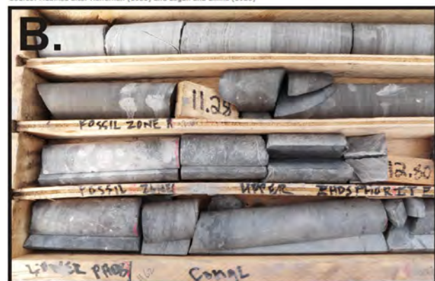
Figure 19. Wapiti East (phosphate) – A. Geology of the Wapiti Lake area. Major fold structures from southwest to northeast include: Red Deer Syncline, Middle Syncline, South Anticline, Wapiti Syncline. Image is from the June 2013 Fertoz Ltd Prospectus; B. Drill core with basal phosphatic conglomerate, upper phosphorite, and fossil zone in the Whistler Member of the Sulphur Mountain Formation.
