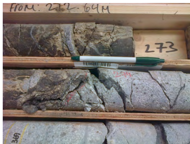
Figure 8. Quartz monzonite porphyry cutting Cache Creek Group, Maggie copper-molybdenum project. (Jim Britton photo)
