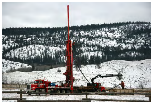
Figure 9. Removing rock cuttings from a rotary drill at the Maggie project where zero-discharge drilling mitigates exploration impacts. (Constantia Resources photo)
