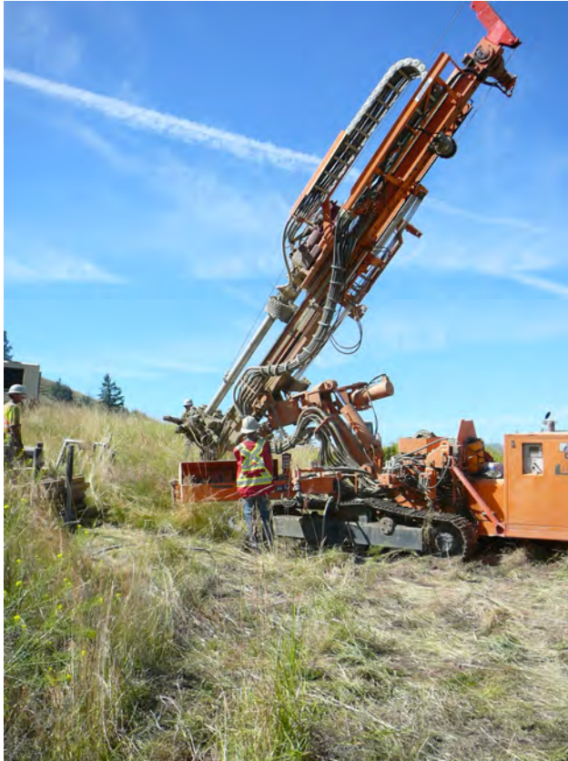
Figure 11. Percussion drill at Sego Resources Inc's Miner Mountain project. (Jim Britton photo)
