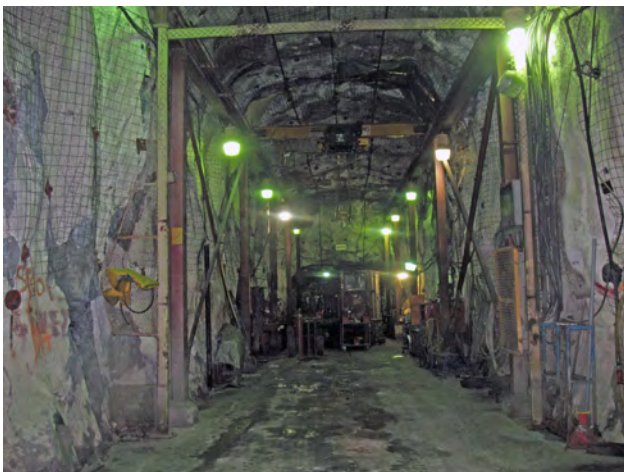
Figure 6. Underground equipment maintenance area at Myra Falls. The mine is in a topographically challenging area surrounded by Class A Park. With limited underground access, mining equipment is assembled and maintained in workshops such as this.
