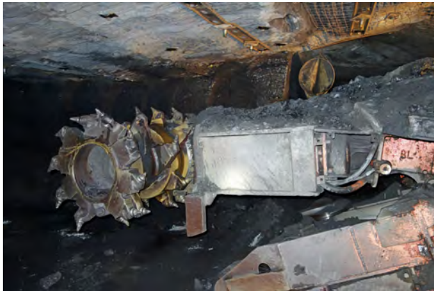
Figure 8. Quinsam Mine uses continuous miners in a room and pillar mining method.
