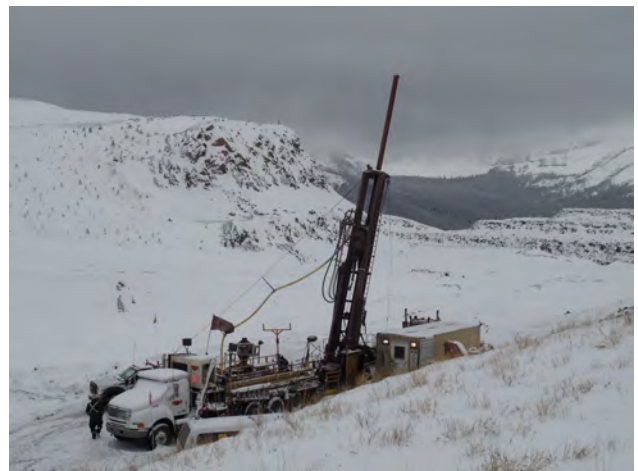
Figure 15. Fall exploration drilling at Coal Mountain (Teck Coal Ltd). The Reverse Circulation drill program targeted the south extension of 6-seam, which is mined in 6-pit.
