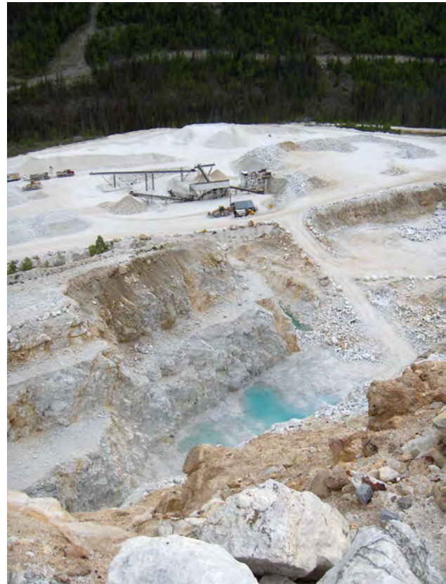
Figure 10. View of the Mount Brussilof mining operations (Baymag Inc). Magnesite is mined from magnesite-rich sparry carbonates of the Cambrian Cathedral Formation. Photo by Dave Grieve.
