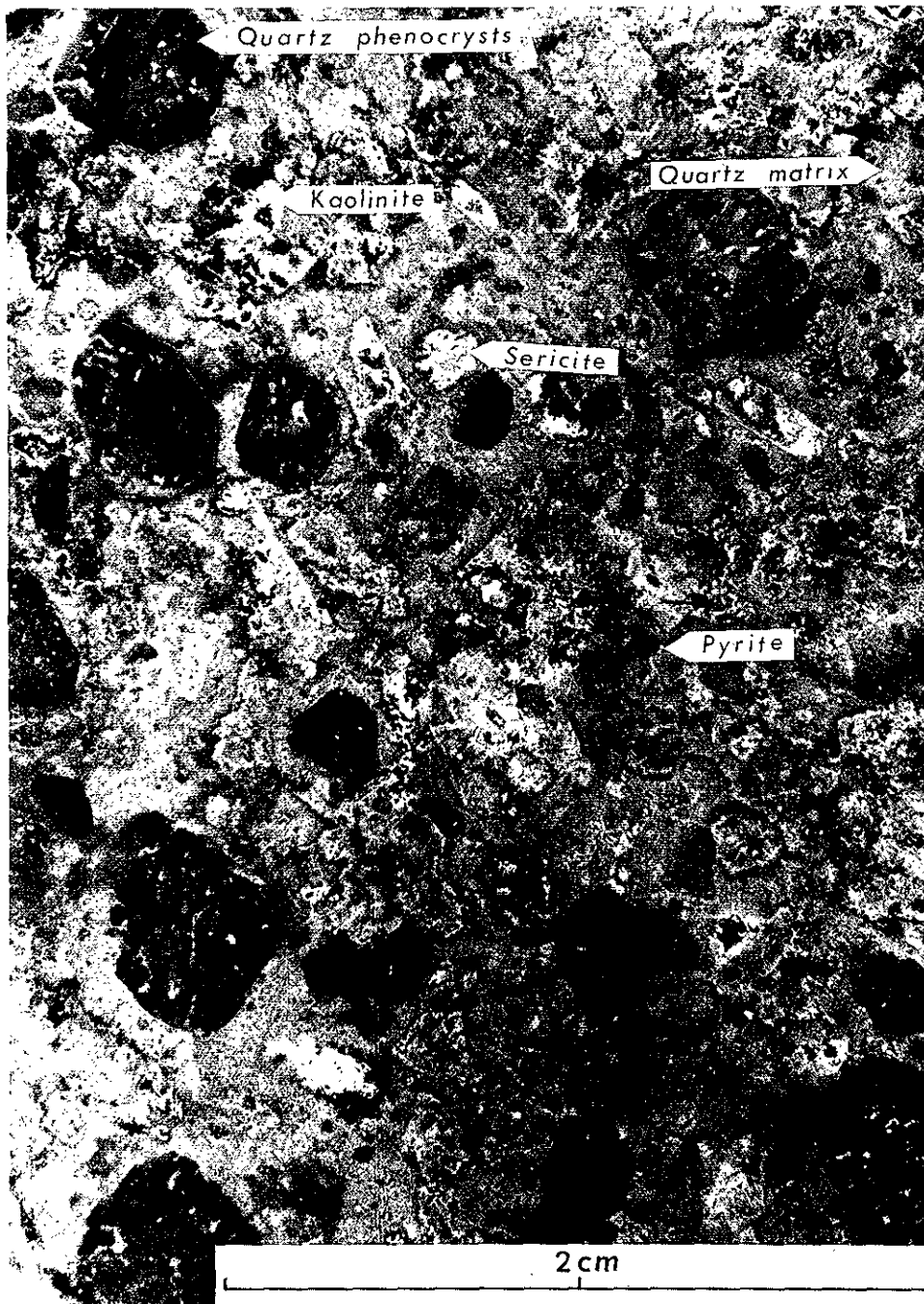
Plate IX. Quartz feldspar porphyry at Island Copper mine. Coarse-grained, rounded, resorbed quartz phenocrysts in a fine-grained quartz matrix containing blebs of sericite and kaolinized feldspar.
