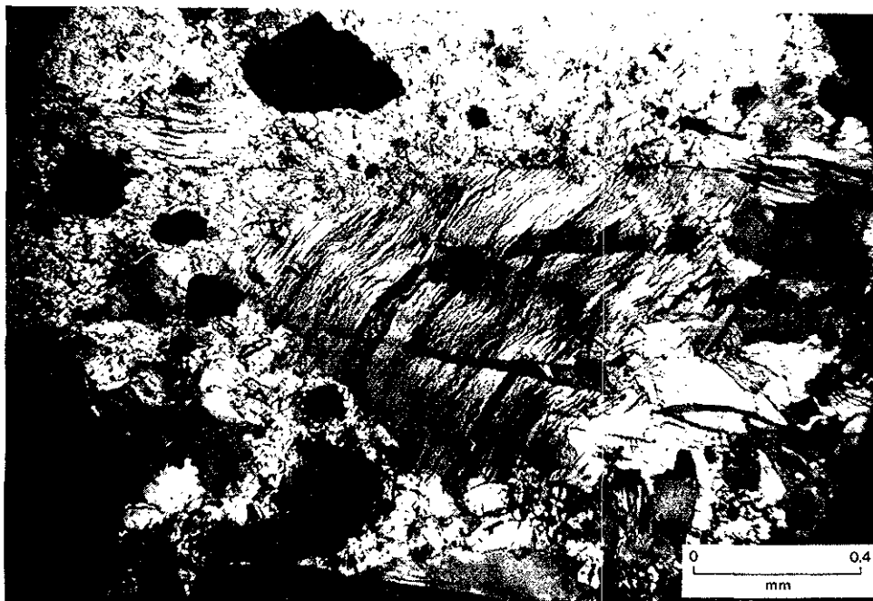
Plate XIVB. Strain slip cleavage in fluorophlogopite with fluorite-filled tension gashes, Rexspar A zone
