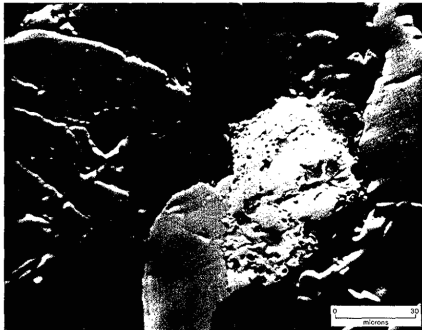
Plate XIII.B. Thorian uraninite grain (light grey) and monzonite (medium grey) in pyrite
