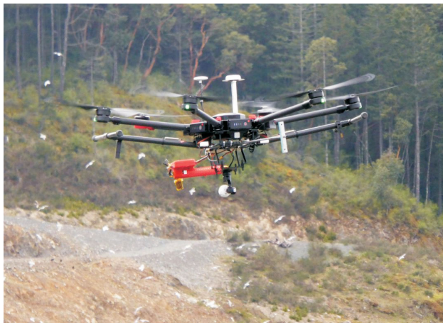
Figure 8. Open-path laser spectrometer on small unmanned aerial vehicle at Hartland Landfill near Victoria, British Columbia.
