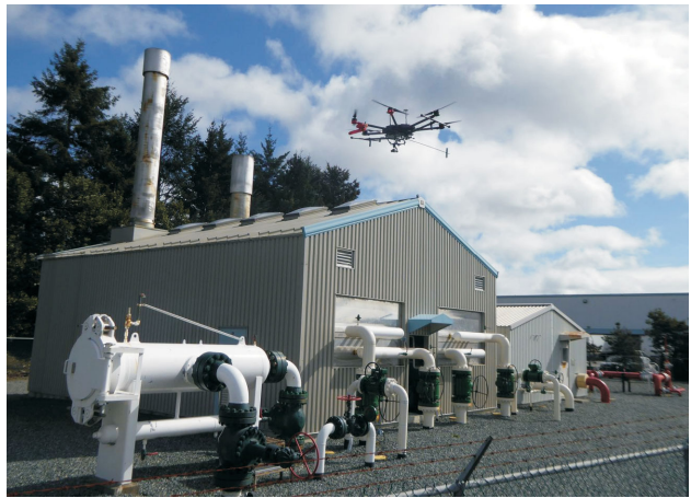
Figure 9. Open-path laser spectrometer on small unmanned aerial vehicle at gas distribution plant in Victoria region, British Columbia.
