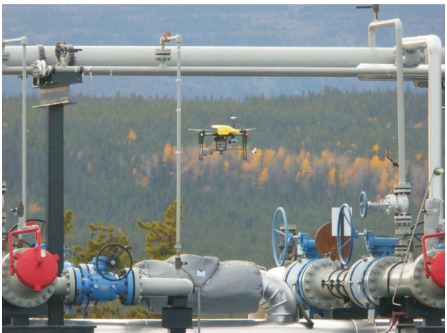
Figure 11. Open-path laser spectrometer on small unmanned aerial vehicle at gas processing plant in Fort St. John region, British Columbia.
