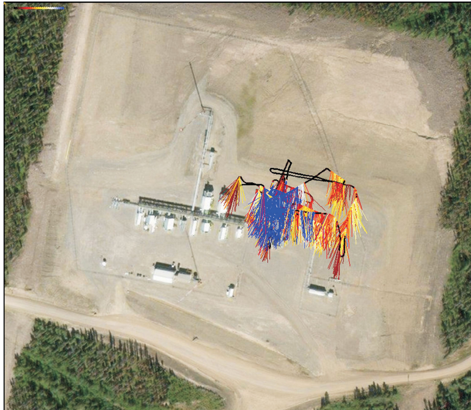
Figure 14. Example of a vector plot of methane emission data collected by an open-path laser spectrometer (OPLS) on a small unmanned aerial vehicle (sUAV) system at a natural gas well pad, near Fort St. John, British Columbia. Methane concentrations are scaled as cooler to hotter colours indicating increasing levels of anomalous methane concentration. The vector lengths indicate the wind direction and speed. The black line is the flight track. Map data: Google, DigitalGlobe.
