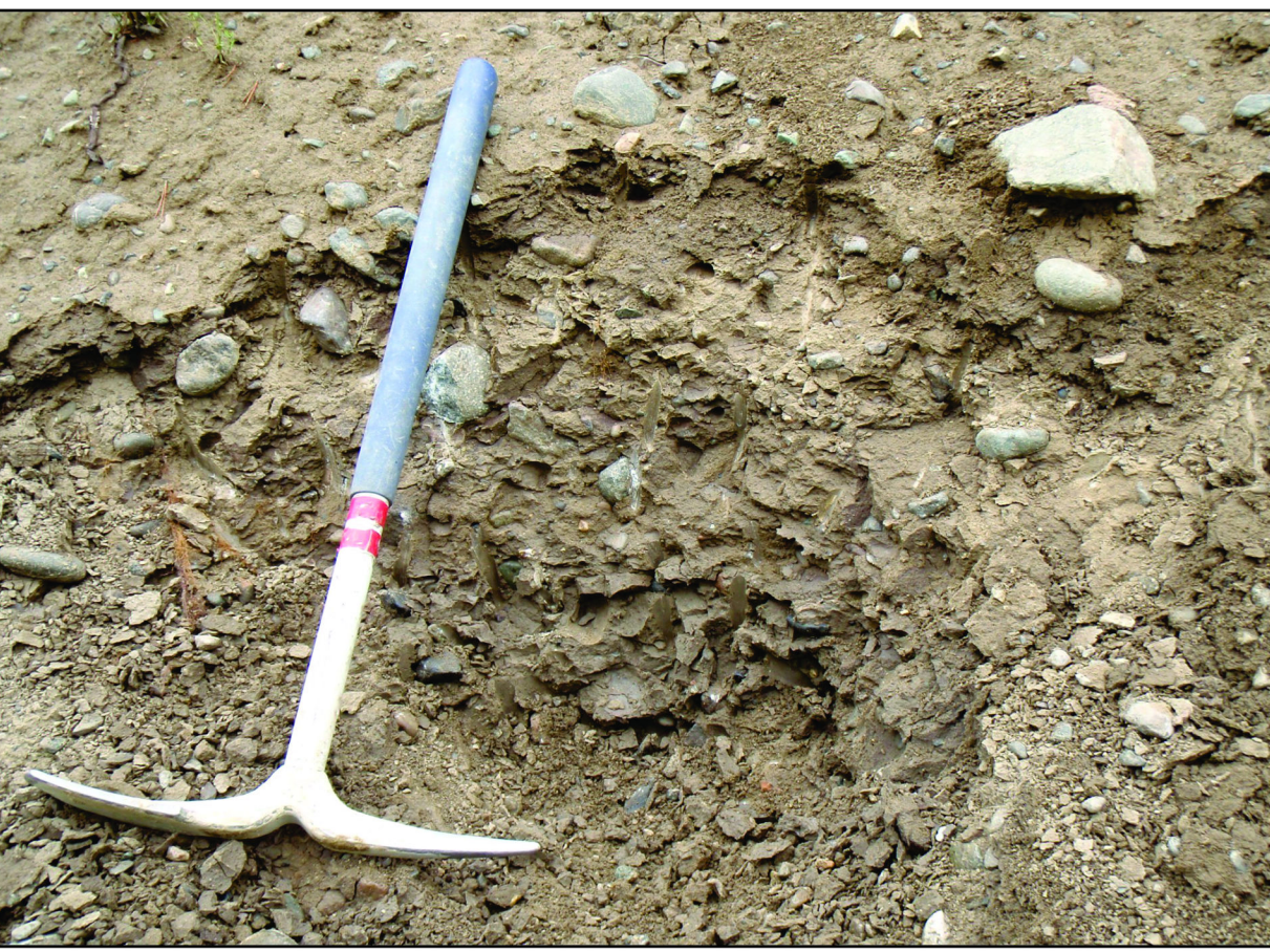
Figure 2. Silt and clay-rich, overconsolidated diamict, interpreted as a basal till. Moderately well-developed vertical jointing and subhorizontal fissility give this till a blocky appearance. Pick for scale (60 cm).
