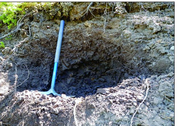
developed vertical jointing and subhorizontal fissility give this basal till a blocky appearance. Pick for scale (65 minesite, at 1400 m asl (locality 1). These rat tails indicate ice-flow toward 272°. Pen for scale (14 cm).
