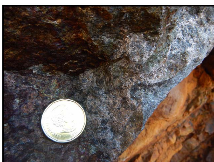
Semi-massive sulphides in peridotite, Pride of Emory orebody.
