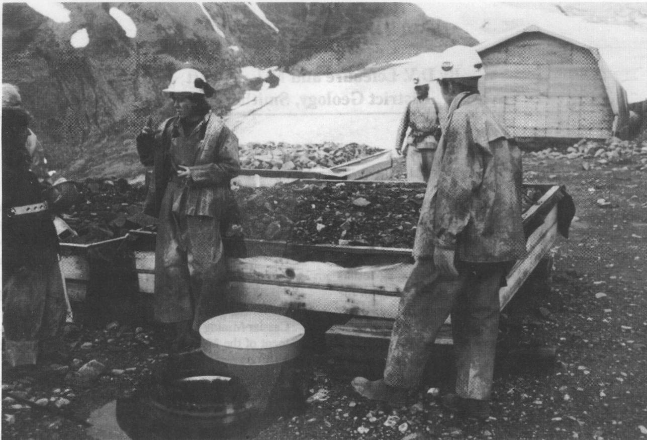
Plate 2-1. Geddes Resources Ltd. continued to work on developing the huge Windy Craggy copper deposit. The company completed numerous studies to assess the impact of a mine in this remote location, including field tests on the potential for developing acid drainage show in the picture above.
