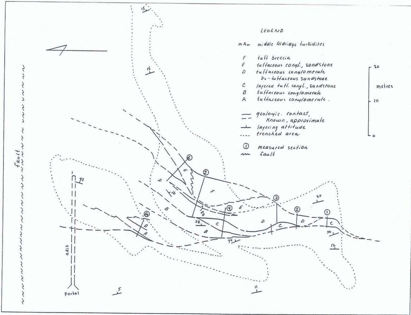
Figure 21. Geological map of the upper fragmental, St. Joe prospect (modified from Pighin, 1983).
