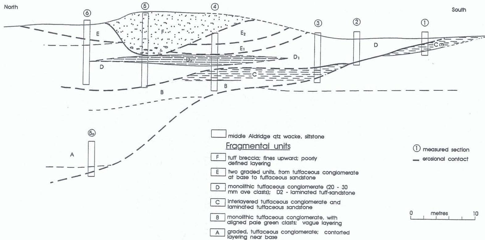
Figure 23. An interpretive section through the upper fragmental, St. Joe prospect.
