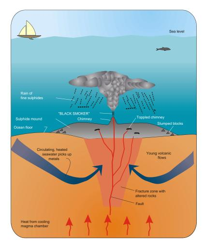
Black smokers are dense, metal rich hot springs on the ocean floor. Ores of base metals are commonly formed on the sea floor along ridges where the earth's plates are spreading apart. The hot, metal-rich fluids are vented through cracks and the metallic minerals precipatate out and build up large deposits as they encounter the cooler, sea water. The ore at Myra Creek formed this way about 380 million years ago.
