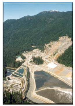
Boliden Westimin's Myra Falls Operations View looking west over HW minesite (lower left) and conveyor belt to mill and water recovery ponds (center). Tailings ponds lower right.
