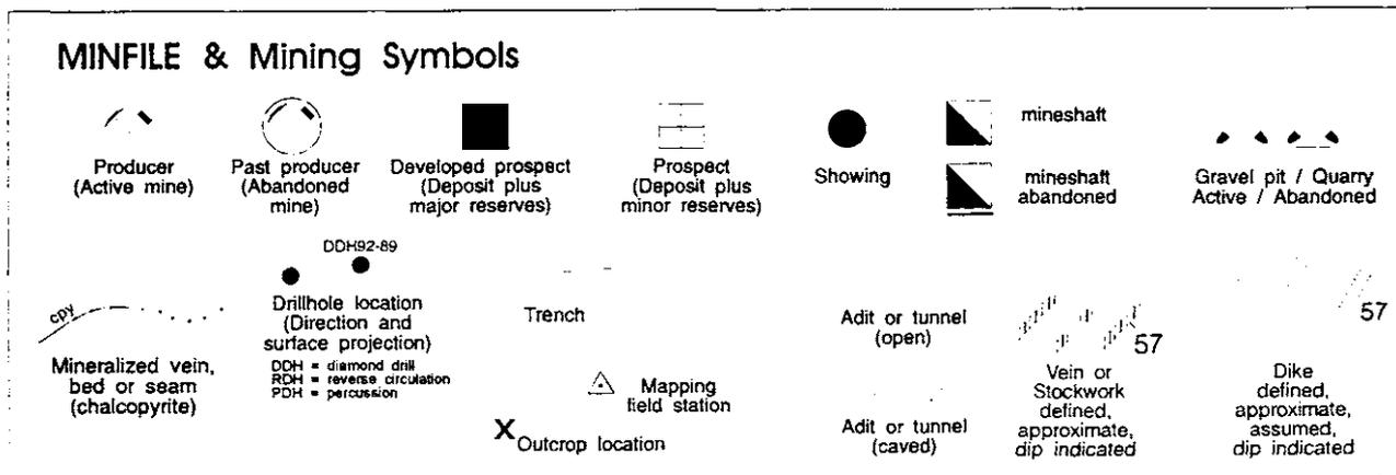
Figure 10. Symbols commonly found on geology maps (modified after Grant and Newell, 1992). Note that surficial geology features are not described in Appendix IX. They are included here only because they are often portrayed on bedrock geology maps. {refer to RIC Surficial Geology mapping standards}
