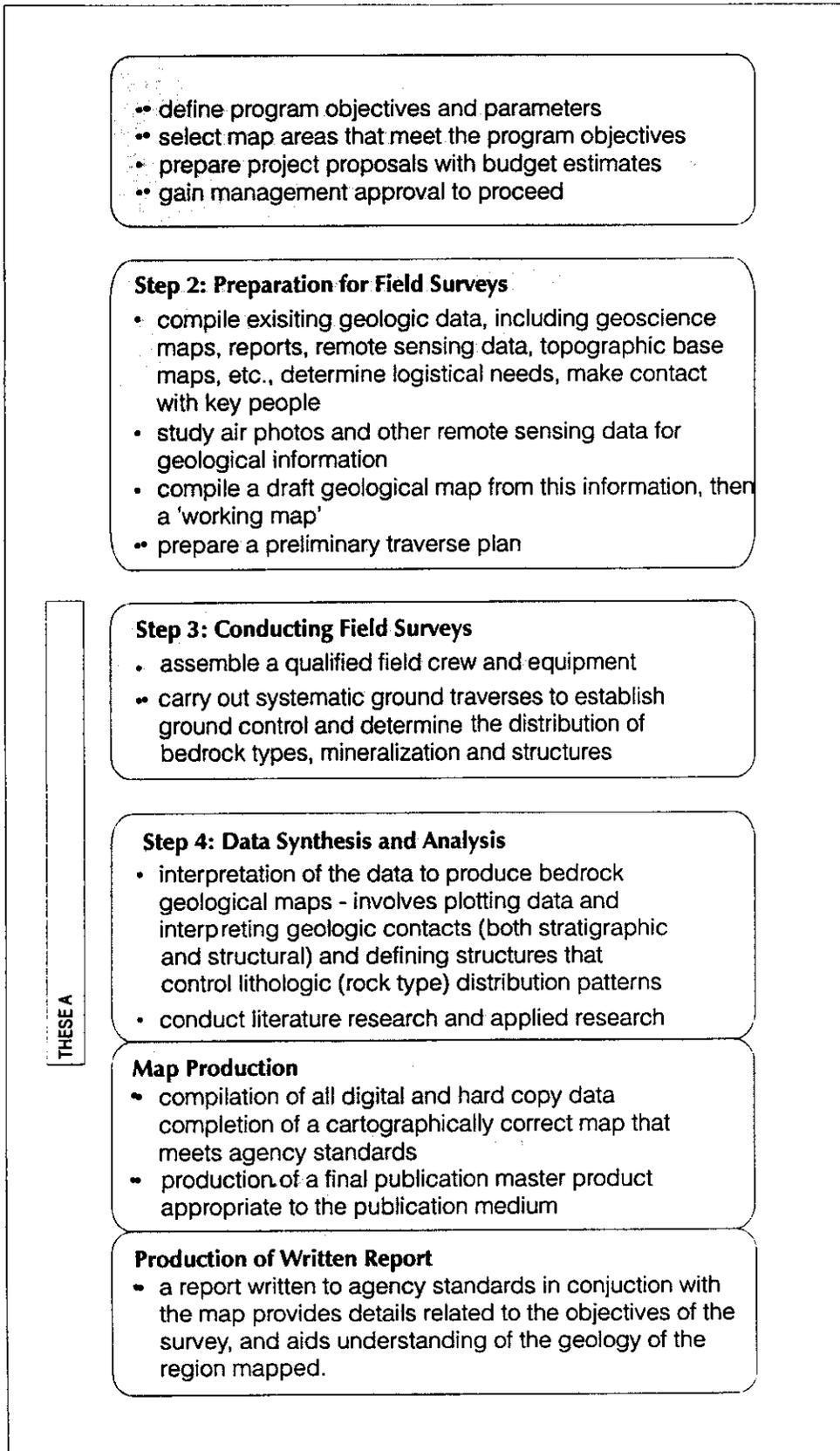
Figure 2. Stages in a bedrock mapping program from inception to final map and report production.
