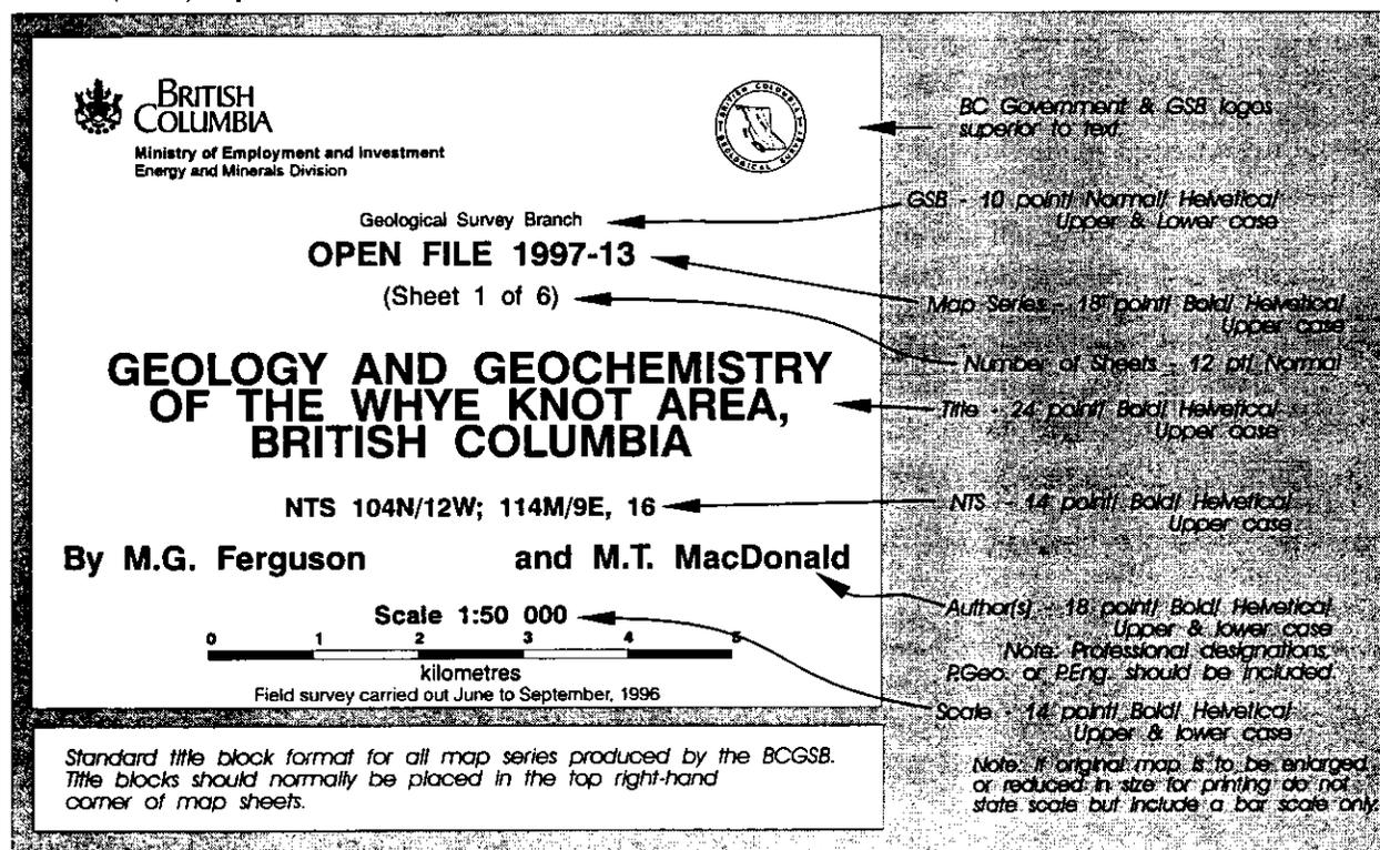
Figure 5. An example of the structure of the title block recommended for use on bedrock maps (that used by the B.C. Geological Survey Branch; from Grant and Newell, 1992)
