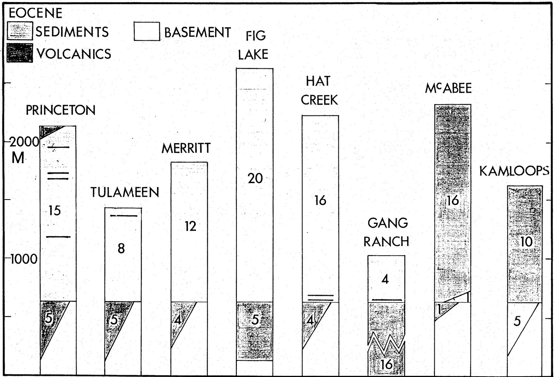
Figure 6: Stratigraphic columns of the Eocene blocks of southern British Columbia showing the thicknesses (in hundreds of metres) of the sediments, waterlain ash (black lines) and volcanics.
