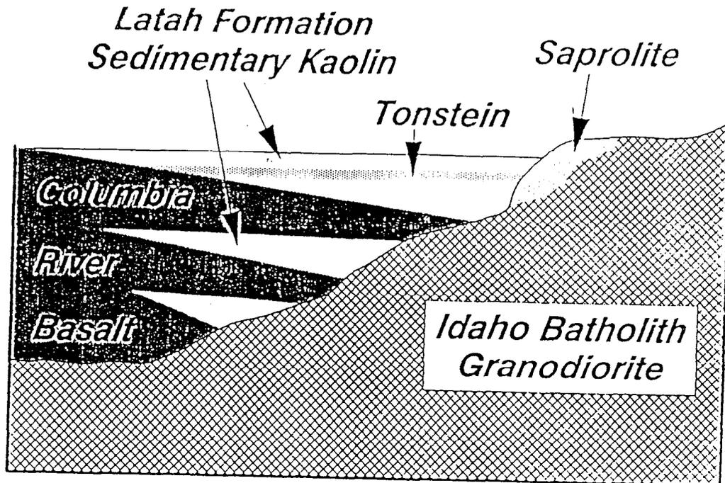
**Figure 5 - Cross-section of kaolin resources in Latah County, Idaho (modified from Ponder and Keller, 1959)**
