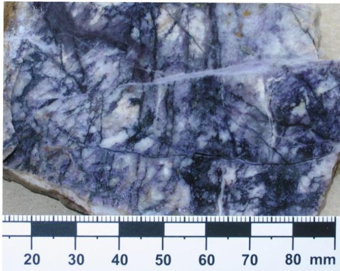
**Figure 6.** Crackle breccia. Dark purple, fine-grained fluorite fills fractures and replaces the pale gray limestone. Rock Canyon Creek deposit, southeastern British Columbia, Canada.
