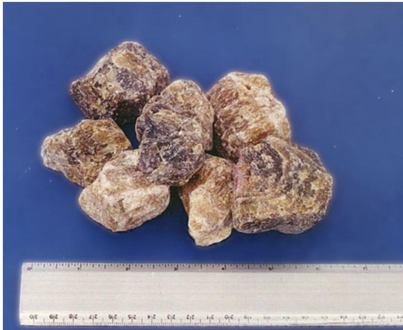
**Figure 13.** Metallurgical grade fluorspar concentrate. The ruler is in inches and centimetres for scale. Photo used with the permission of the MEXICHEM.
