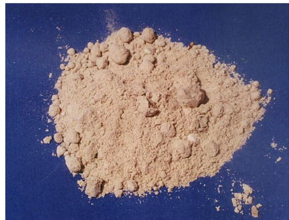
**Figure 12.** Acid grade fluorite concentrate; particles are less than 1 mm in size. Photo used with the permission of MEXICHEM.
