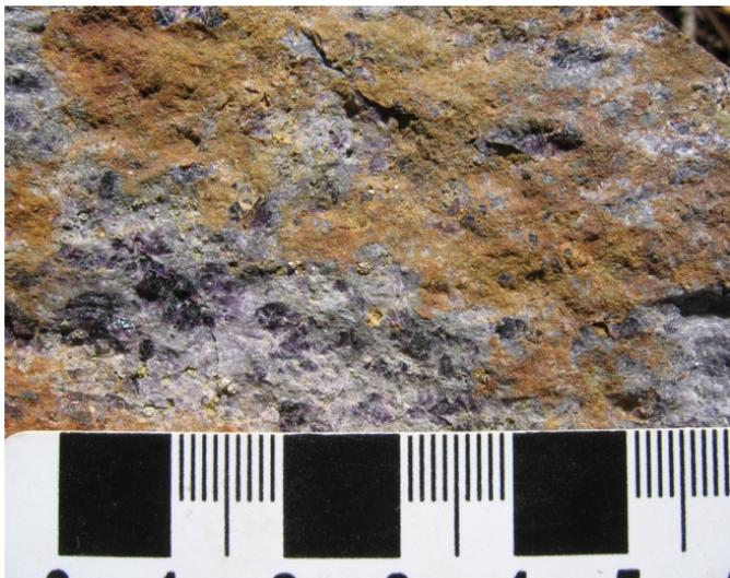
**Figure 7.** Fluorite disseminated in trachytic meta-tuff, Rexspar deposit, central British Columbia, Canada. Fluorite is purple to almost black. Weathered sulphides give the rock a rusty-brown appearance (fine division on the scale = 1mm).
