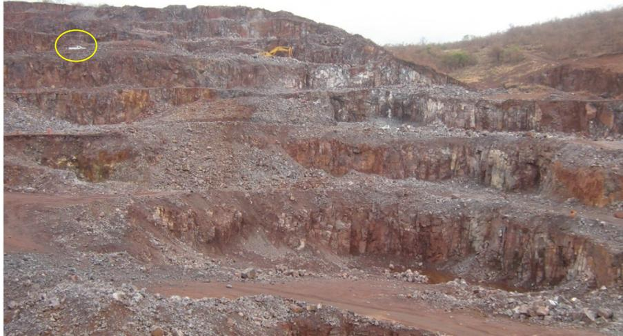
**Figure 11.** Large open pit fluorite mine, within the giant Vergenoeng fluorite – iron oxide - fayalite pipe, South Africa. Pick-up truck for scale (circled). Photo used with permission of Vergenoeg Mining Company Ltd.
