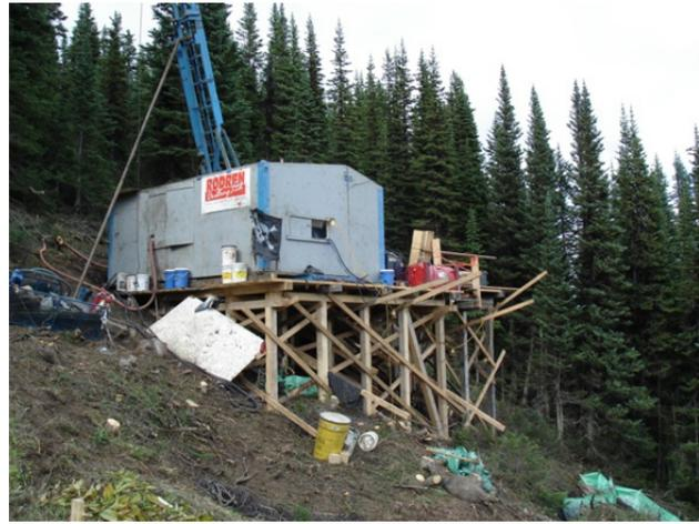
Figure 26. Akie, large drill platform to support a drill rig for deep holes.
