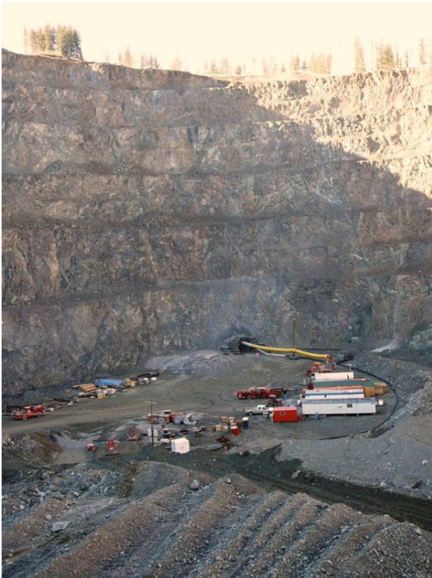
Figure 29. The bottom of the Wight pit at the Mount Polley copper-gold mine was used to start a decline to facilitate testing the Boundary and Zuke zones where the potential for underground mining is being considered.
