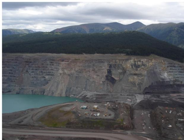
Figure 8. Kemess South mine showing failures on the north wall that result from graphite-bearing Asitka Group sedimentary rocks. A basement “high” of Takla rocks separates tailings in the West pit from active mining in the East pit.
