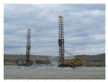
**Fig. 8.** Blast-hole drilling for Phase 2 mining in the MBX pit, Mt. Milligan mine.
