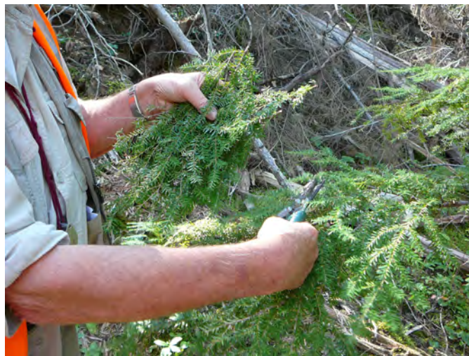
Fig. 9. At the TL project, Mabel Lake area, biogeochemistry helps find massive Pb-Zn sulphides in dense forest with no outcrop.
