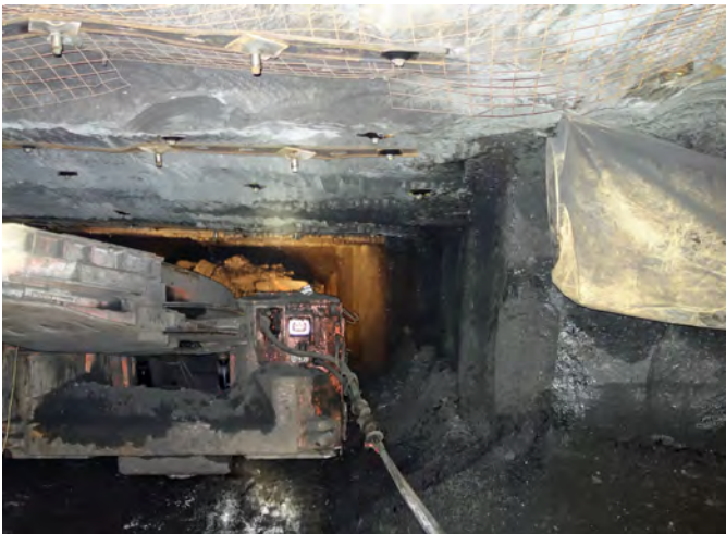
Fig. 8. Operator's view from the back of a continuous miner at Quinsam Coal.
