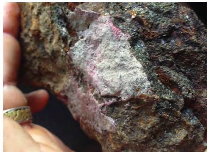
Fig. 14. Nickel bloom field test for nickel sulphide at a discovery on the Lekcin property north of Hope. Photo by Chris Paul.
