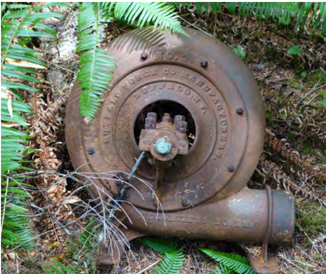
Fig. 13. A forge blower at abandoned workings on the Pacific Iron property, probably dating to 1916.
