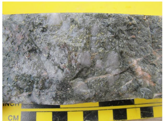
**Fig. 13.** Kemess East chalcopyrite-pyrite mineralization with magnetite-quartz-biotite-chlorite alteration in brecciated Black Lake monzodiorite unit (KH-15-23).
