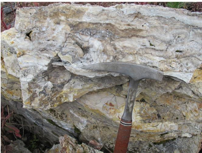
**Fig. 11.** Crustiform-colloform banded chalcidonic quartz vein with comb texture and lattice bladed quartz in vugs at 2 X Fred.
