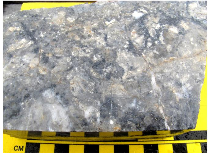
**Fig. 10.** Slabbed quartz vein grab sample from Lawyers with gold-silver bearing sulphide mineralization.
