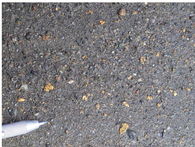
**Fig. 9.** Gold with heavy minerals from a sluice box capture mat at a Manson Creek placer mine.
