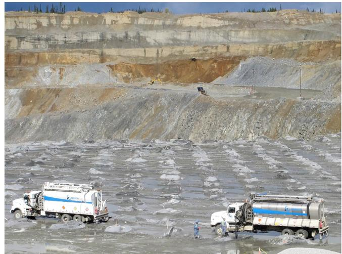
**Fig. 5.** Emulsion trucks on blast pattern in the 66 Zone at Mt. Milligan mine. View is looking north.
