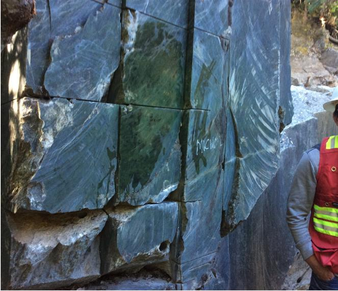
**Fig. 21.** Previously sawed bedrock exposure to be bulk sampled using expanding grout at Pishon Green Jade.
