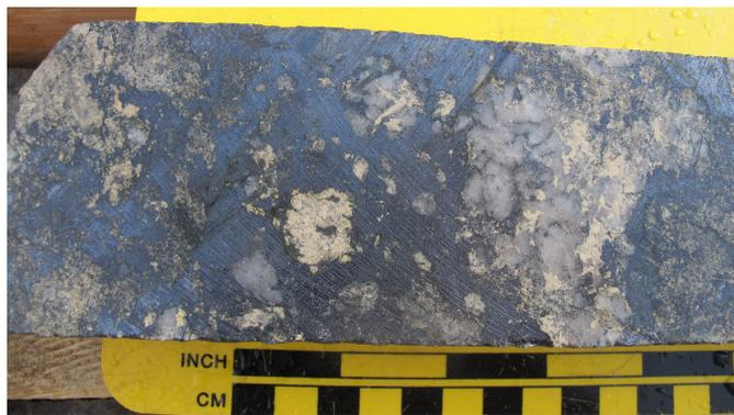
**Fig. 16.** Supergene chalcocite replacement mineralization in the Kwanika Central Zone (K-16-177).
