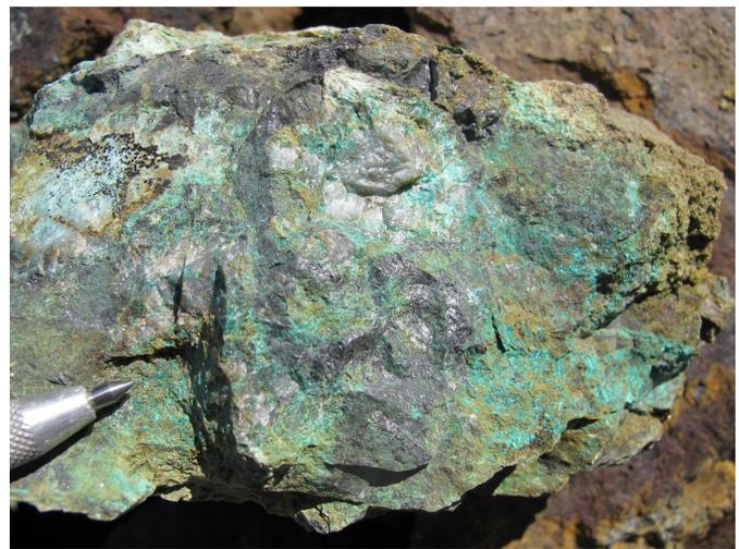
**Fig. 15.** Malachite-stained sample from the No. 1 magnetite vein on the Cat property.
