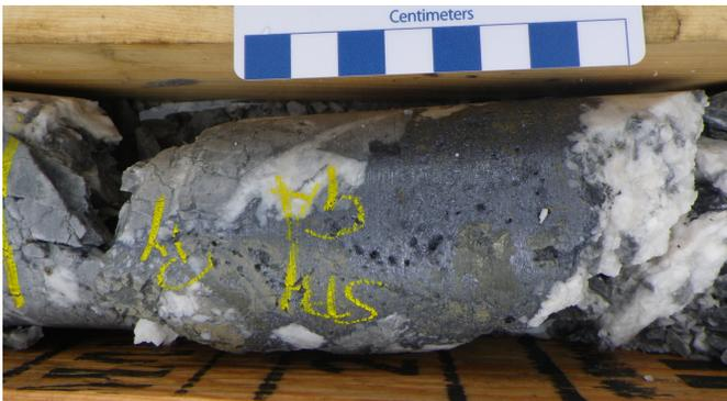
**Fig. 13.** Indy project, hole IB18-009, 79 m, galena, sphalerite and pyrite in quartz, Black Stuart Group.
