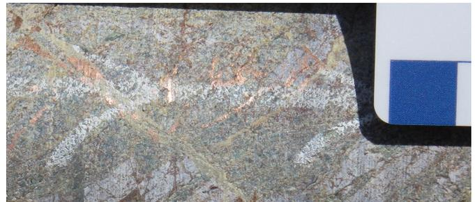
Fig. 10. Kwanika project, hole K-18-181, 317.5 m, native copper in supergene zone monzonite. Scale in cm.
