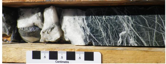
**Fig. 8.** Snowbird project, hole SB-18-03, 45 m, shear zone with stibnite in quartz stockwork.
