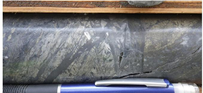
**Fig. 7.** Gibson project, hole G18-10, 62.8 m, late-stage very fine grained quartz-sulphide veinlets (dark grey) cutting mineralized Takla Group host rock.
