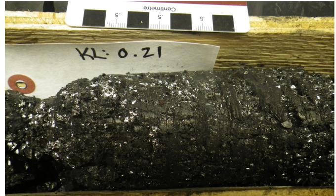
Fig. 15. Panorama North project, hole PNDH-18-04, 63 m, fractured anthracite coal.
