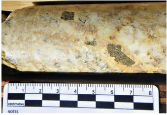
Fig. 5. Wicheeda project, DDH WI19-21, 57 m, REE-mineralized carbonatite.
