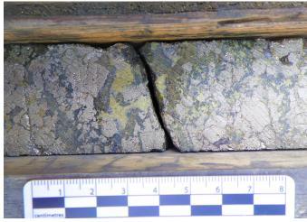
**Fig. 4.** Stardust project, DDH 19-SD-430P, 579 m, chalcopyrite and pyrite.
