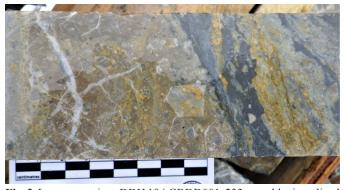
**Fig. 3.** Lawyers project, DDH 19AGBDD001, 233 m, gold mineralized silica-flooded hydrothermal breccia.
