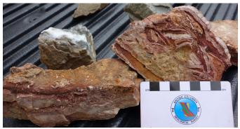
**Fig. 4.** Epithermal textures (crustiform quartz, chalcedony veining) in hand specimens collected in Talisker Resources Ltd.'s regional exploration of the Spences Bridge belt.
