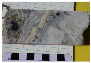
**Fig. 2.** Quartz, chalcedony and adularia veining with ginguro (black) in lapilli tuff at Westhaven Ventures Inc.'s Shovelnose project.
