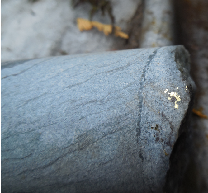
Fig. 4. Visible gold in drill core (NQ size). Photo courtesy of Apex Resources Inc.
