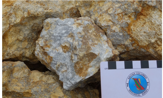
Fig. 3. Teeta Creek, hydrothermal breccia with intensely clay altered felsic volcanic clasts in a chalcedonic matrix.
