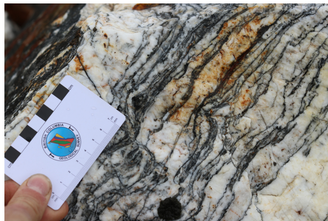
Fig. 4. Gold-bearing quartz vein with pyrite and tourmaline stylolites; from tailings at Table Mountain, Cassiar Gold project.
