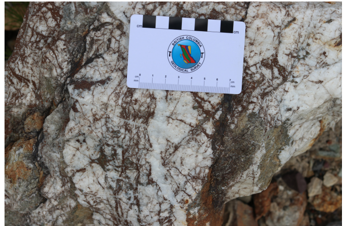
Fig. 3. Ore-grade 'Boulder' quartz vein with disseminated sulphides and Fe-carbonate stringers at Dome Mountain.
