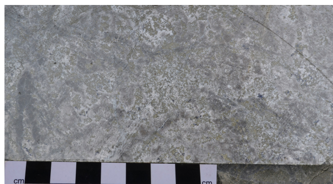
Fig. 4. Silica-clay-pyrite is one of the principal alteration types at Hushamu. This sample has disseminated chalcopyrite and minor bornite.
