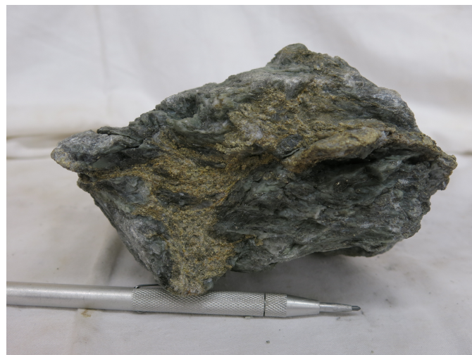
Fig. 2. Gold (present as electrum) in quartz-sericite-pyrite altered fine-grained lapilli tuff at Brucejack.
