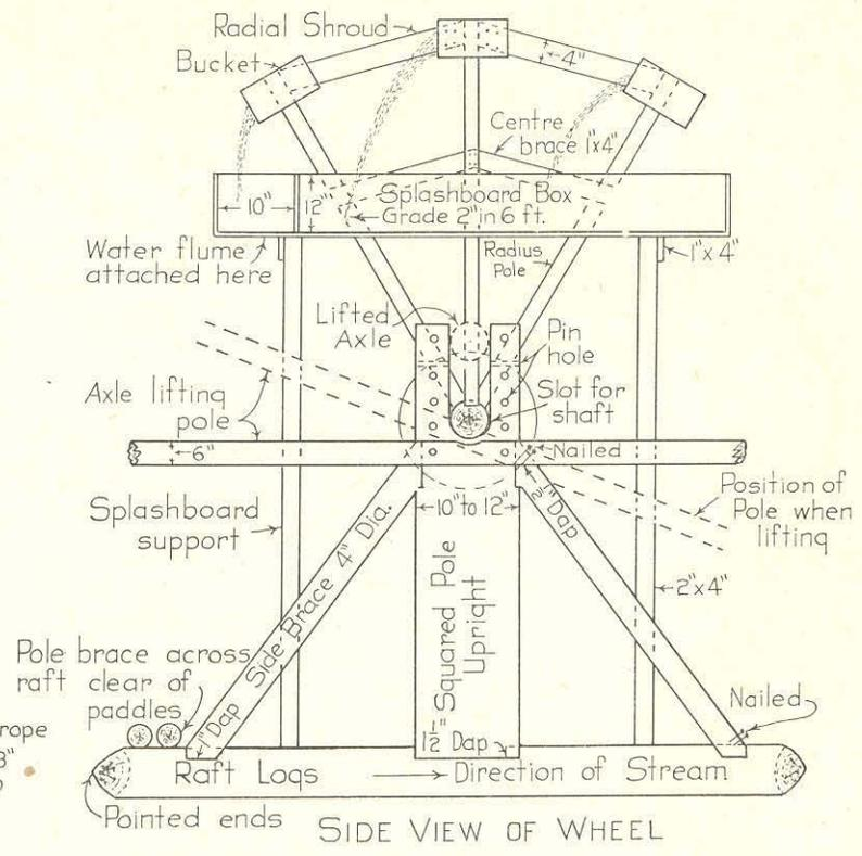
Sections showing Construction of Parts of Undercurrent-wheel.
