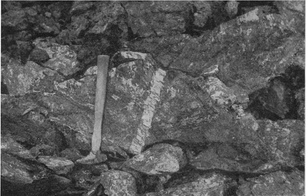
Vein of high-grade asbestos at open-pit mine of Cassiar Asbestos Corporation Limited, McDame Creek.
