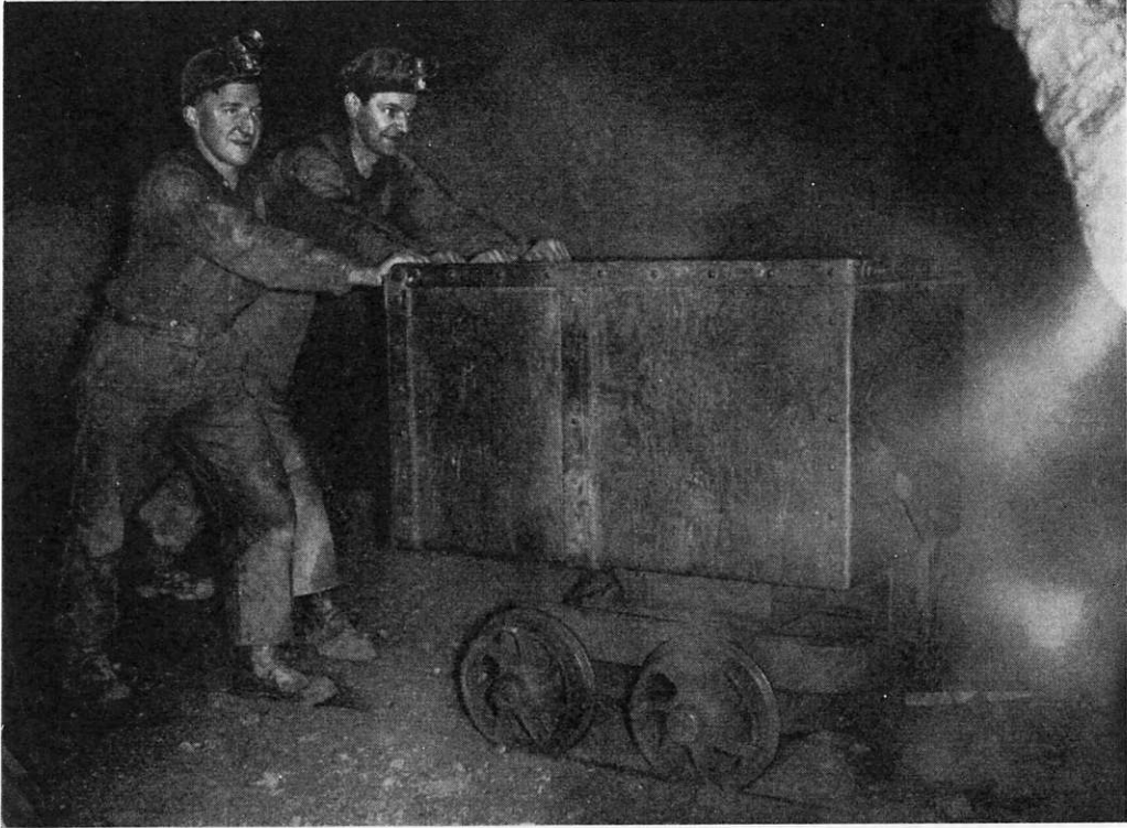
Hand-tramming ore underground in a small mine.
