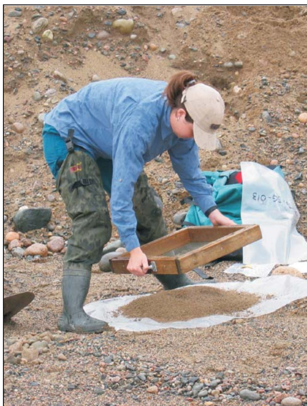
Figure 2. Sieving coarse grained sand and gravel for kimberlite indicator minerals.
