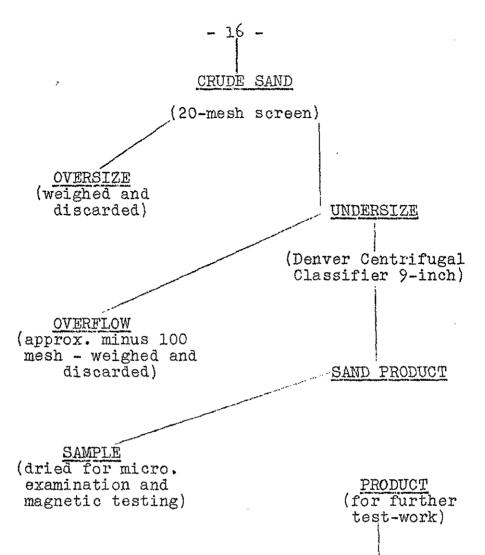
The classifier was so adjusted that the required separation was effected with minimum water and maximum agitation. By so doing it performed the dual role of sizing and washing.
