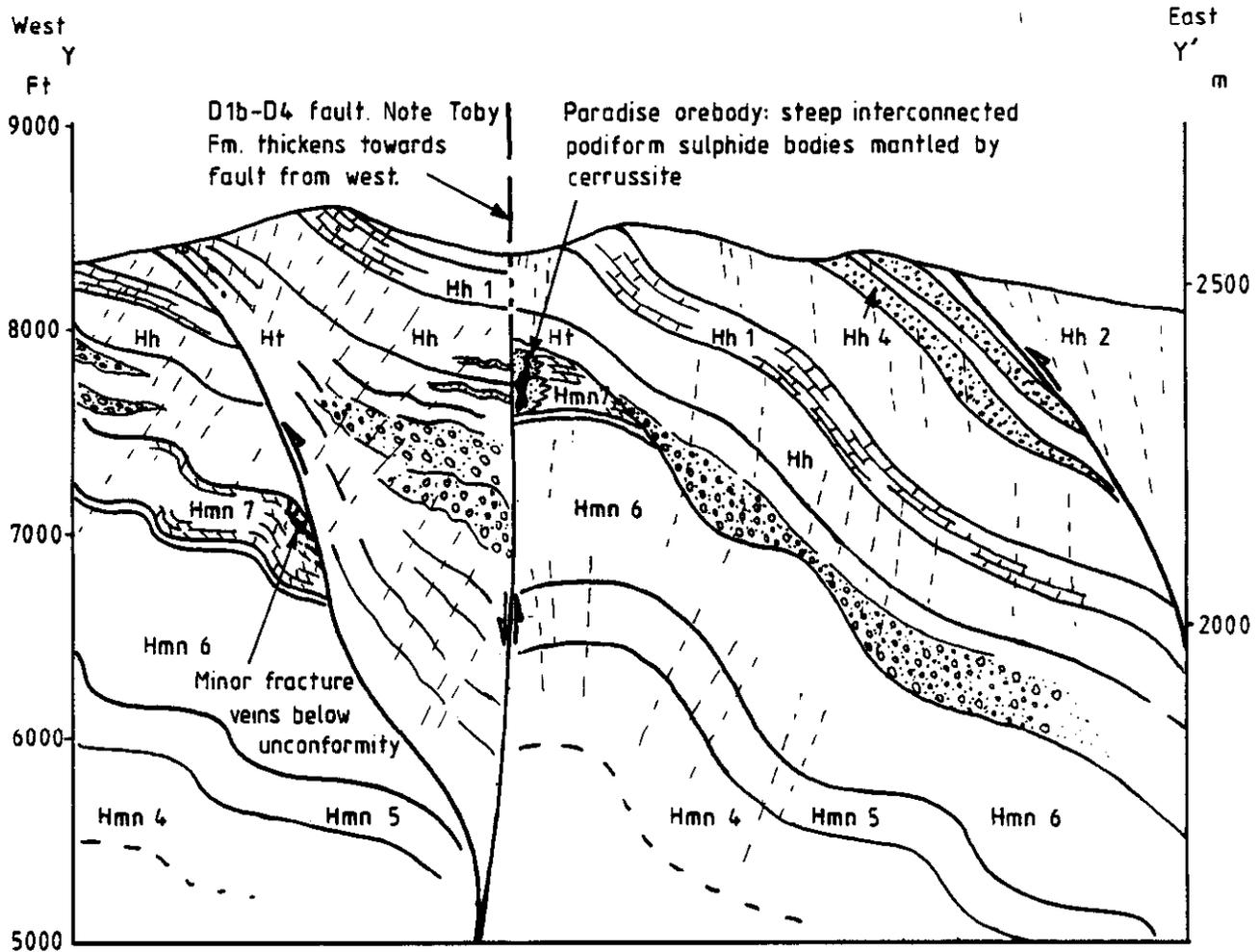
Figure 17b. Geological cross section of the Paradise mine.
