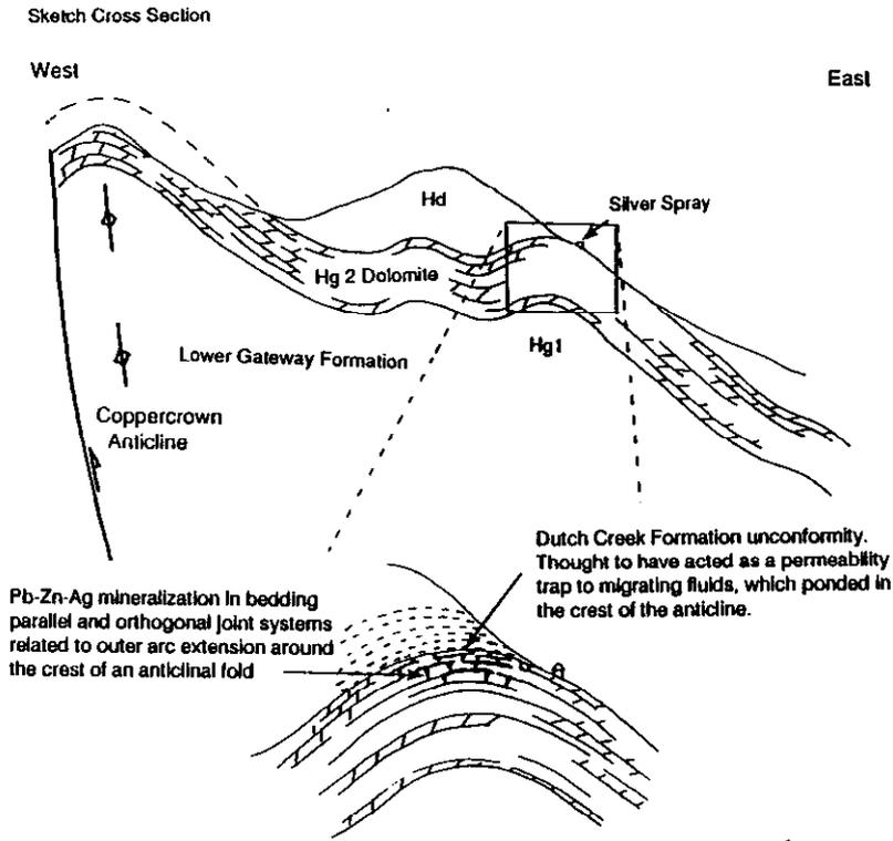
Figure 26b. Cross section of the Silver Spray mine.
