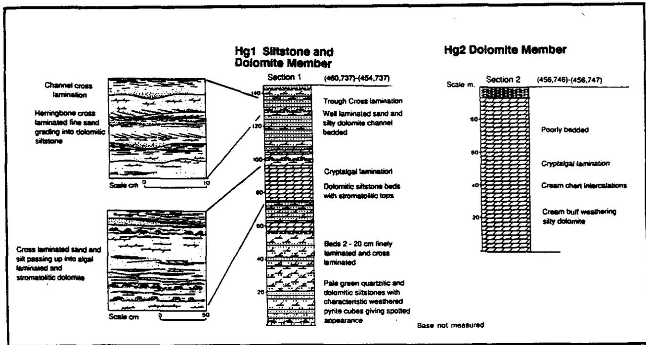
Figure 5. Sections 1 and 2 - Measured section of the Lower Gateway Formation.
