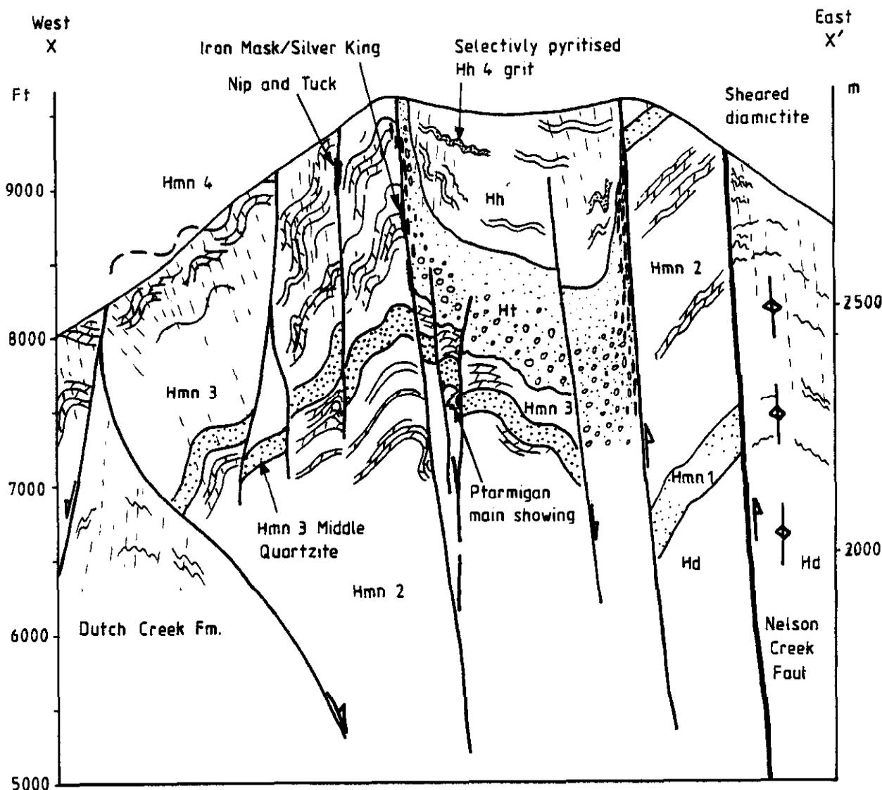
Figure 19b. Geological cross section of the Ptarmigan group of mines.
