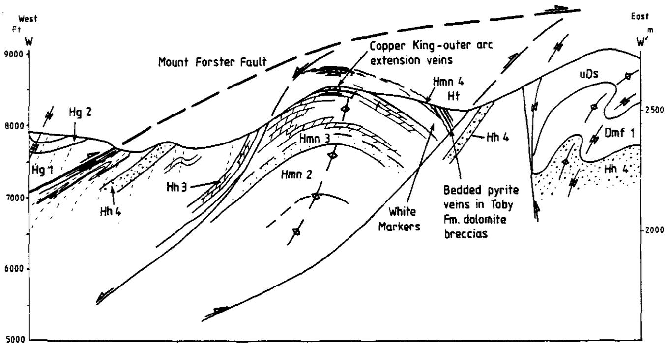
Figure 25b. Geological cross section of the Copper King mine.
