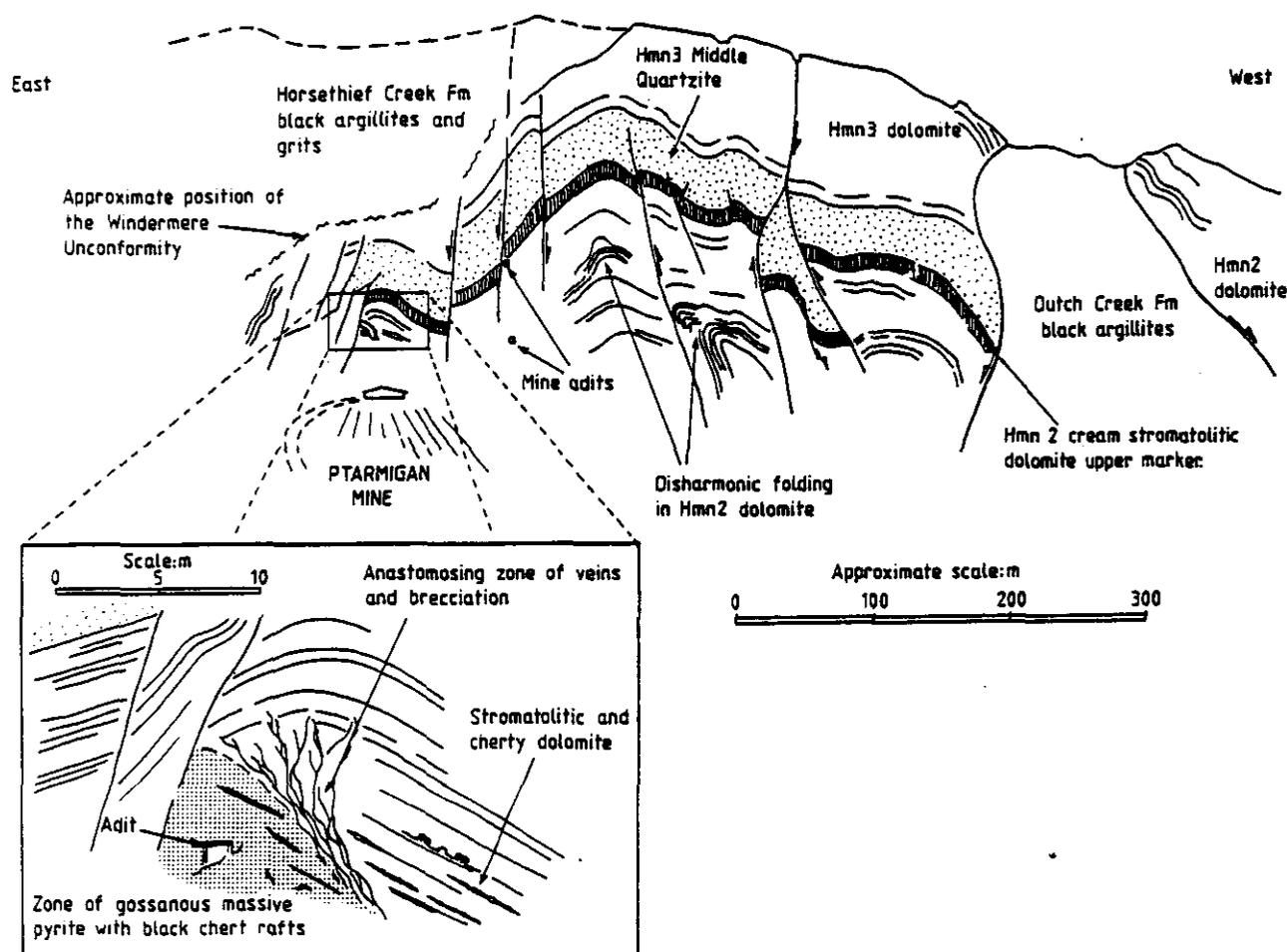
Figure 20. Field sketch of the Ptarmigan mine.
