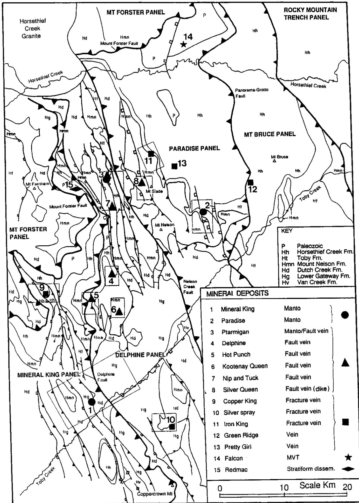
Figure 14. Summary geological map showing location of mineral deposits and areas of detailed prospect mapping referred to in the text. (Note: detailed maps for 7, 12, 13 and 15 are not included in this report.)
