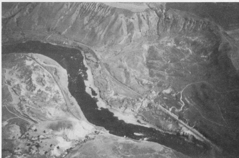
Figure 19: Aerial view of 1888 Ashcroft landslide. The landslide involved approximately 15 million cubic metres of Pleistocene glaciolacustrine sediments and blocked the Thompson River (flowing to bottom right) for 44 hours.
