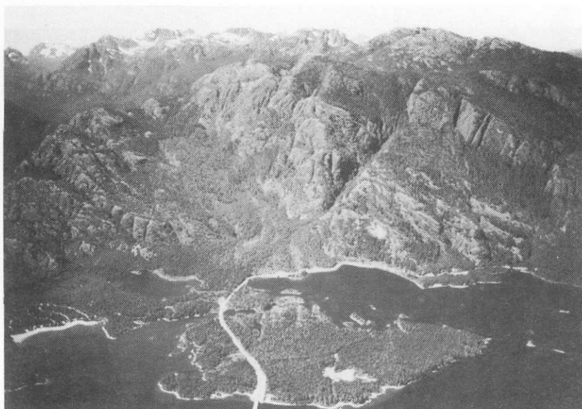
Figure 2: Oblique aerial view of the prehistoric Buttle Lake rock avalanche, Vancouver Island (see Fig. 1 for location). The rock avalanche is one of several on Vancouver Island involving volcanic rocks of the Karmutsen Formation.
