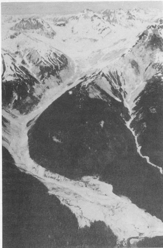
Figure 18: Aerial view of 1975 Devastation Glacier debris avalanche. The landslide involved 13 million cubic metres and originated in altered Pleistocene pyroclastic rocks on the western flank of Pylon Peak. The landslide killed four people.
