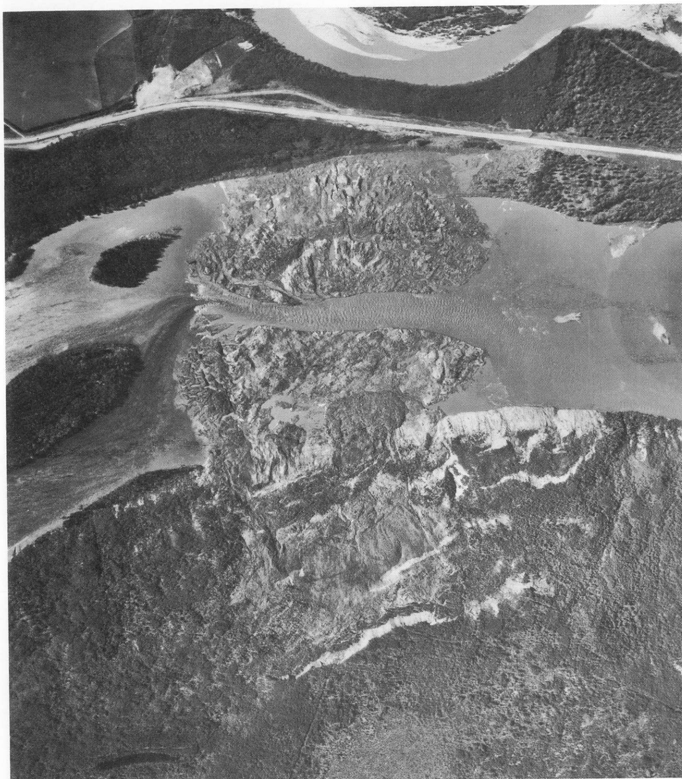
Figure 20: Vertical aerial photograph of 1973 Attachie landslide (BC5529-075). The landslide involved approximately 24 million cubic metres of Pleistocene glaciolacustrine sediments and temporarily blocked the Peace River.
