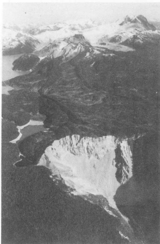
Figure 11: Aerial view of The Barrier, a steep rock face formed by the successive failure of the margin of the Clinker Peak lava flow, the most recent failure being the 1855-56 rock avalanche. Clinker Peak is visible as the obvious source of the lava flow. Mount Garibaldi is visible in the right background.
