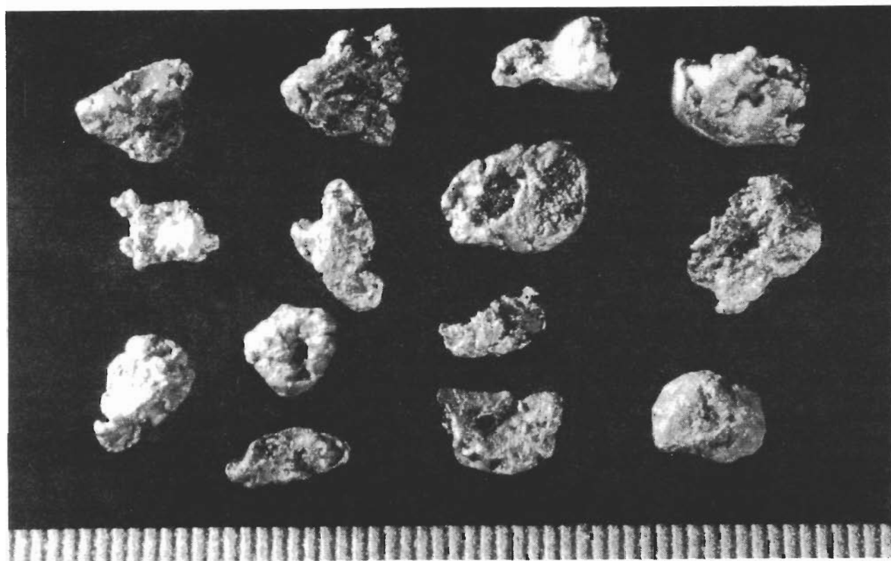
Plate 2. Irregular, chunky gold particles from Sugar Creek (108). Scale at bottom of photograph in tenths of millimetres.
