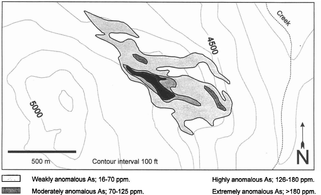
Figure 10. Arsenic soil anomaly for the Silver 1 property. Modified after Richards (1986).
