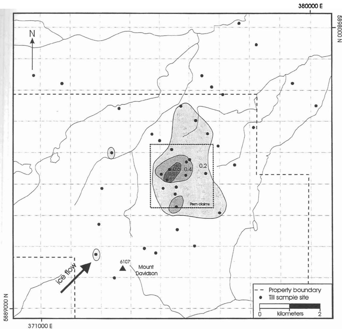
Figure 29: Till dispersal anomaly pattern for silver (Ag), contoured at 0.2, 0.4 and 0.6 ppm, Blackwater-Davidson claims.
