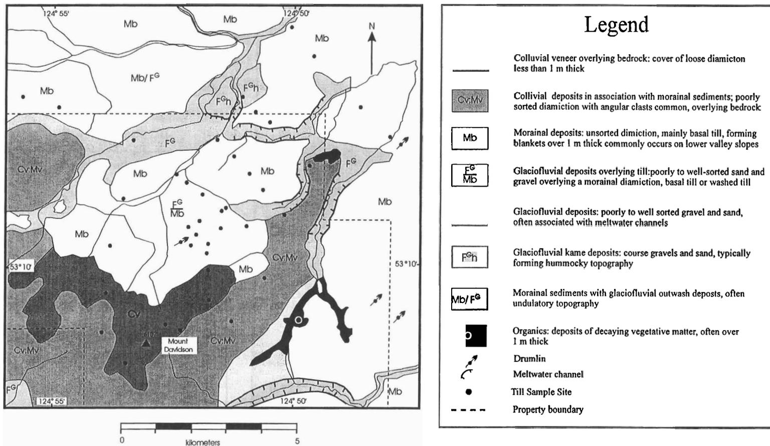
Figure 22: Surficial geology of the Blackwater-Davidson claims (adapted after Giles and Levson, 1995).
