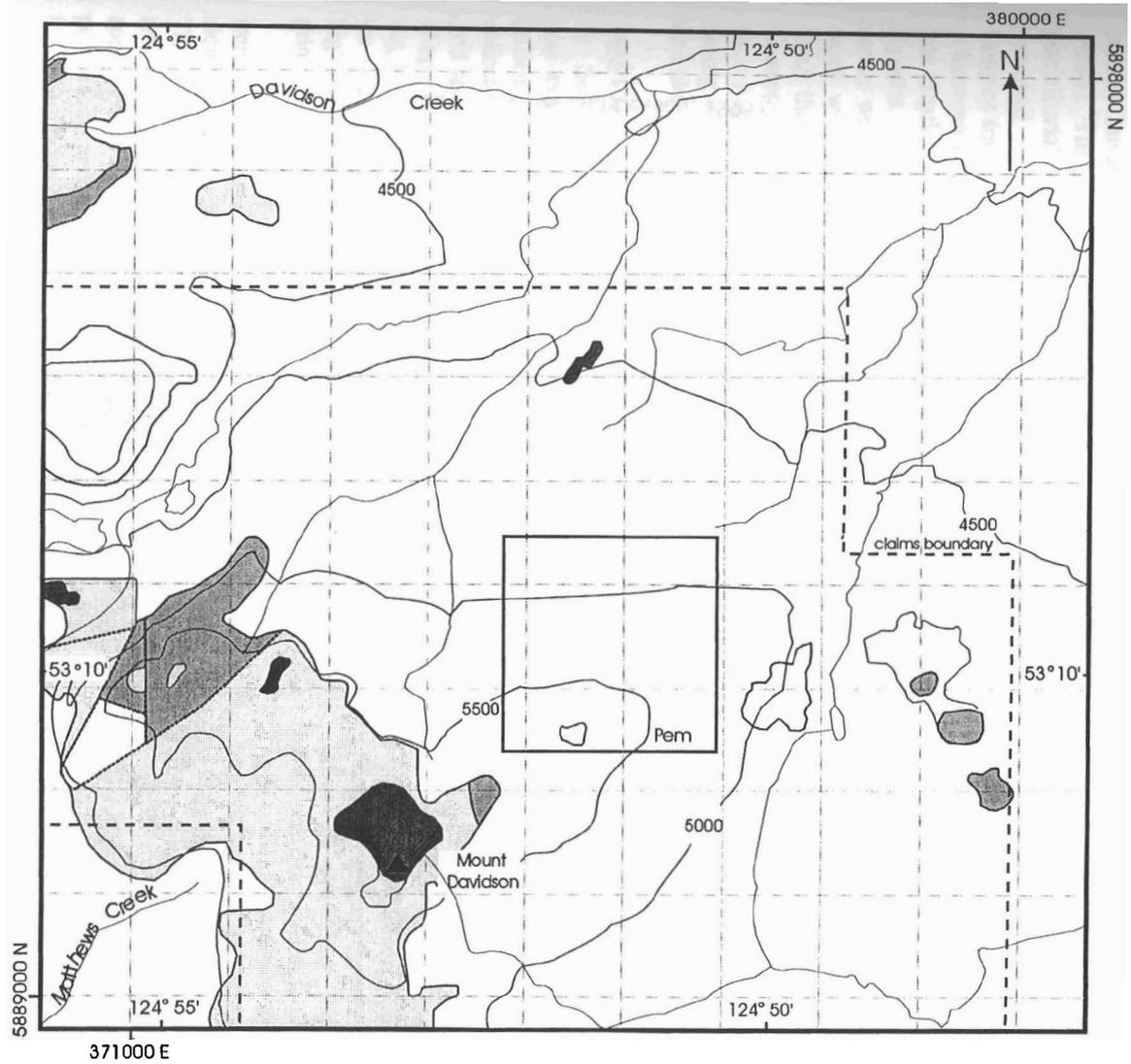
Figure 21: Bedrock geology of the Mount Davidson area (After Diakow *et al.*, 1995a).
