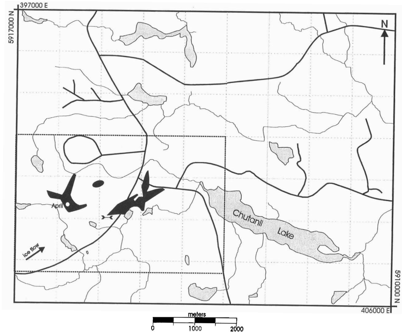
Figure 9: Soil dispersal pattern for lead (Pb) over 28 ppm, dark pattern on the CH claims (Edwards and Campbell, 1992).
