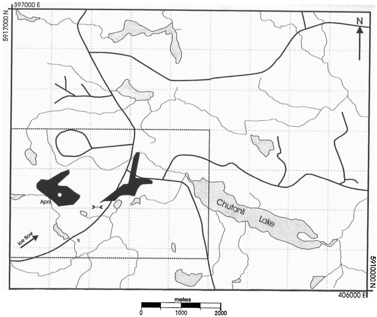
Figure 10: Soil dispersal pattern for zinc (Zn) over 120 ppm, dark pattern on the CH claims (after Edwards and Campbell, 1992).
