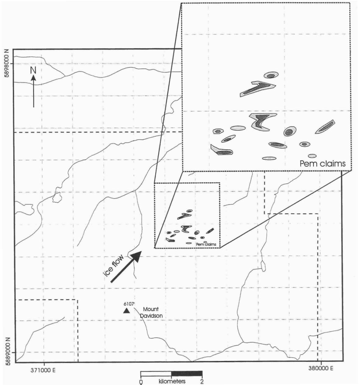
Figure 23: Anomalous soil pattern for gold (Au), contoured at 50 and 100 ppb, Blackwater-Davidson claims (Allen, 1992).
