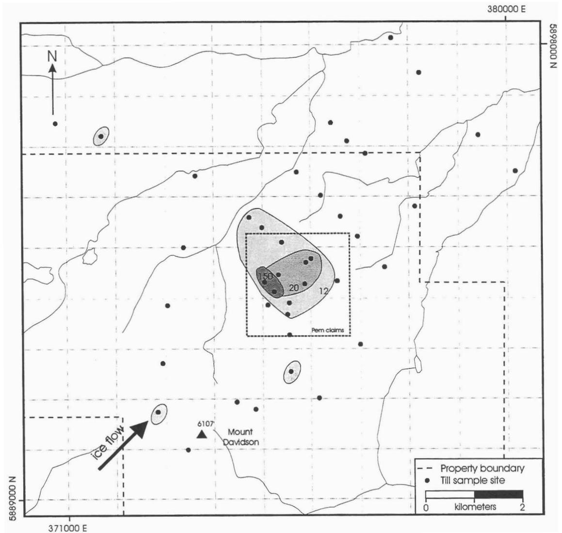
Figure 30: Till dispersal anomaly pattern for arsenic (As), contoured at 12, 20 and 150 ppm, Blackwater-Davidson claims.
