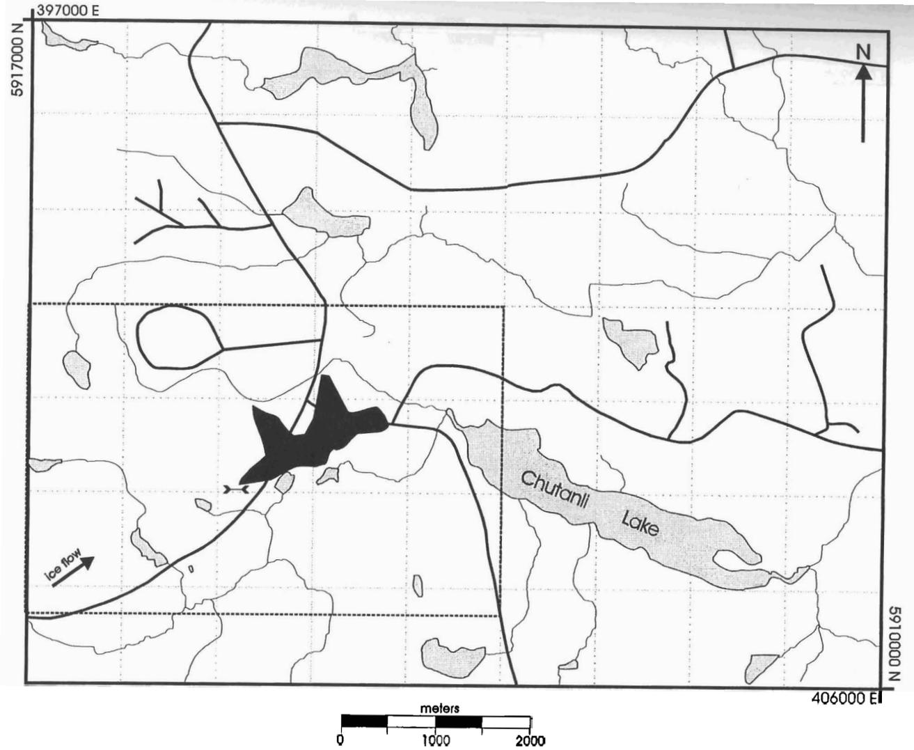
Figure 8: Soil dispersal pattern for copper (Cu) over 82 ppm, dark pattern on the CH claims (Edwards and Campbell, 1992).
