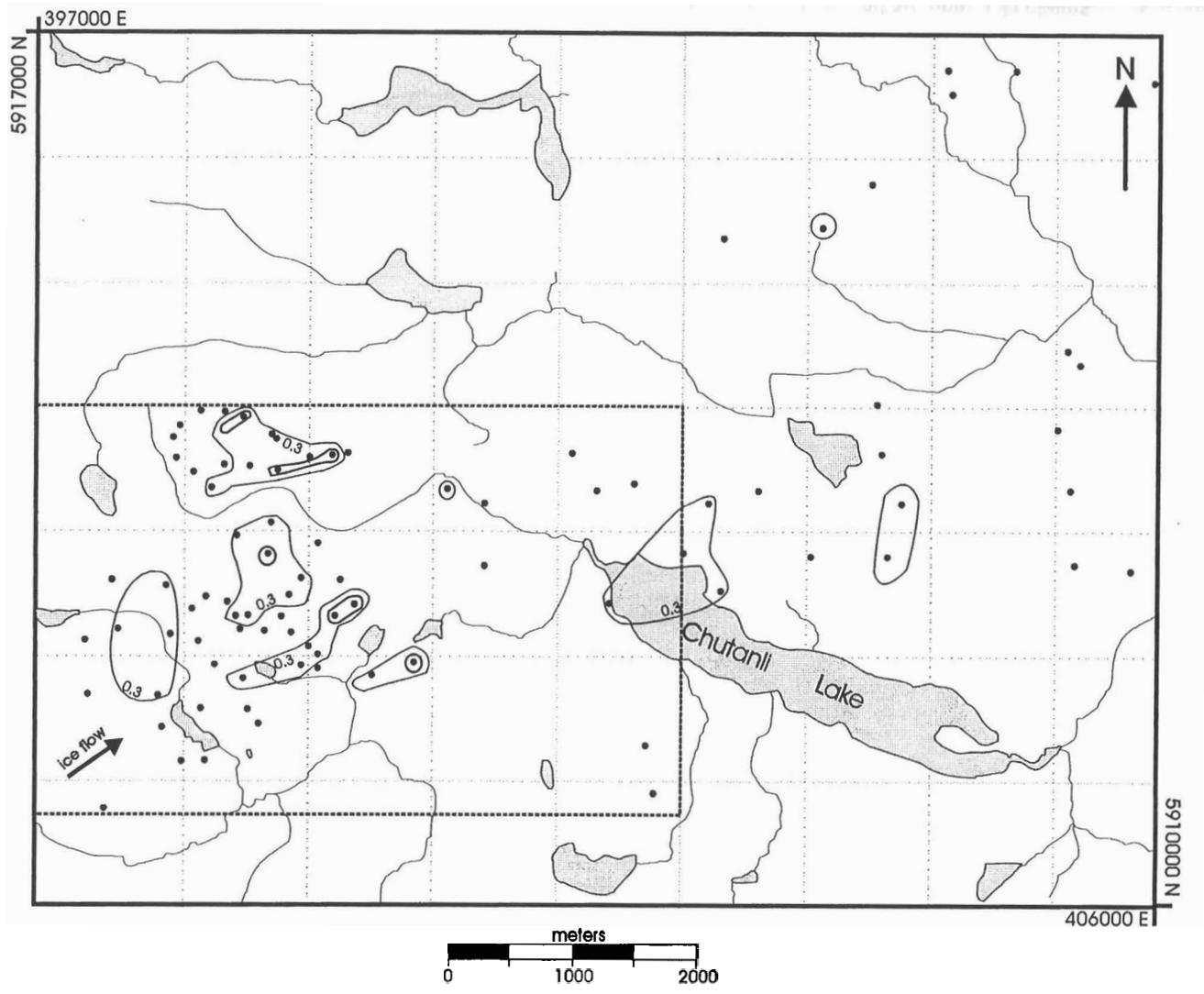
Figure 16: Till dispersal anomaly pattern for silver (Ag), contoured at 0.3 and 1 ppm, CH claims.
