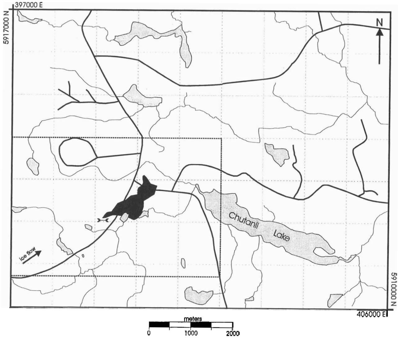
Figure 7: Soil dispersal anomaly pattern for gold (Au) over 6 ppb, dark pattern on the CH claims (Edwards and Campbell, 1992).
