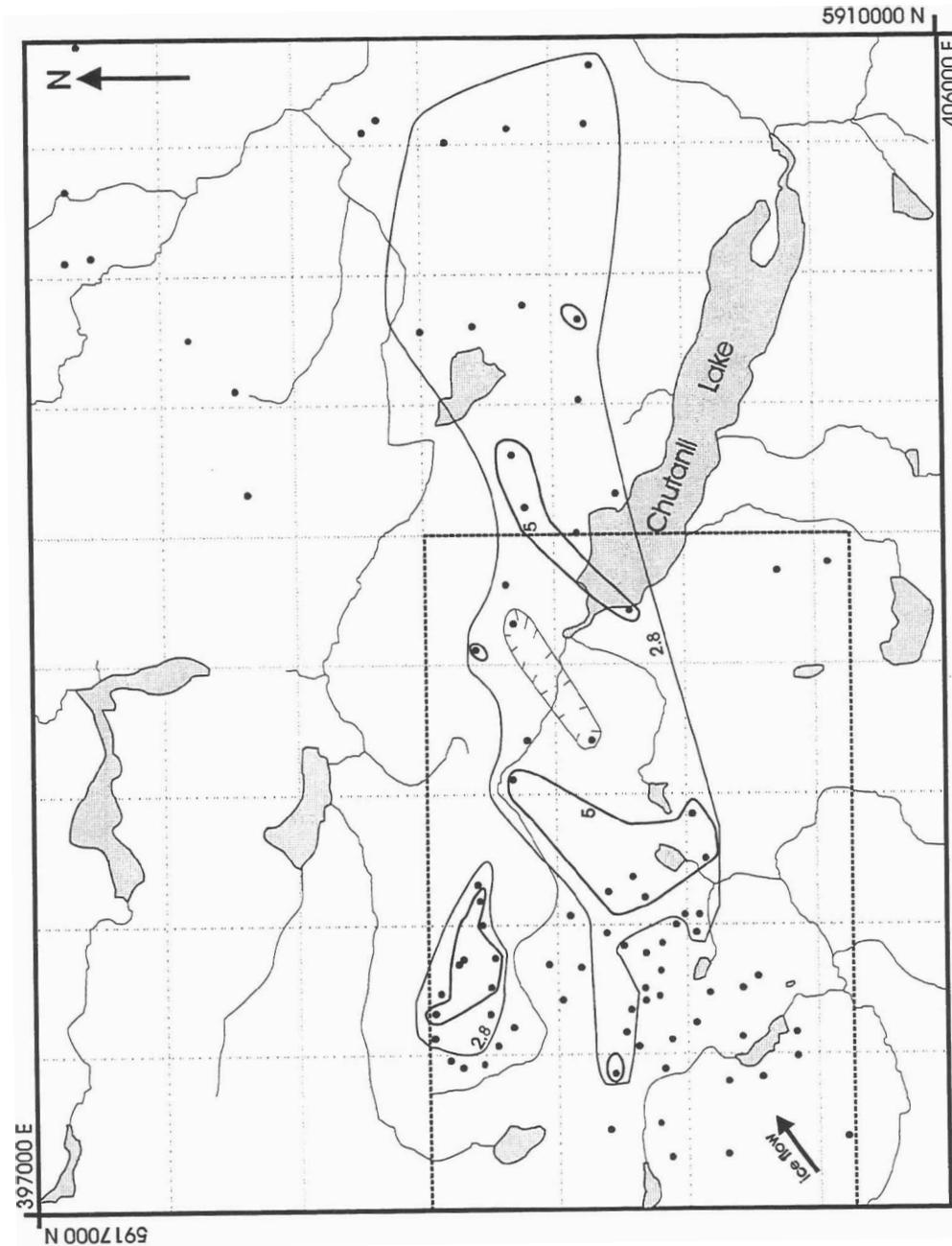
Figure 19: Till dispersal anomaly pattern for antimony (Sb), contoured at 2.8 and 5 ppm, CH claims.
