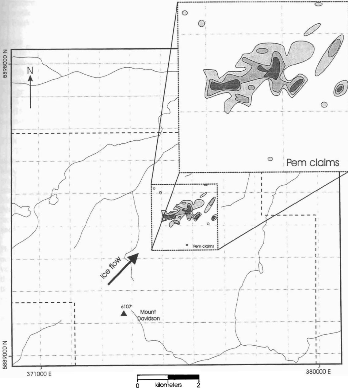
Figure 24: Anomalous soil pattern for silver (Ag), contoured at 1, 2 and 5 ppm, Blackwater-Davidson claims (Allen, 1992).
