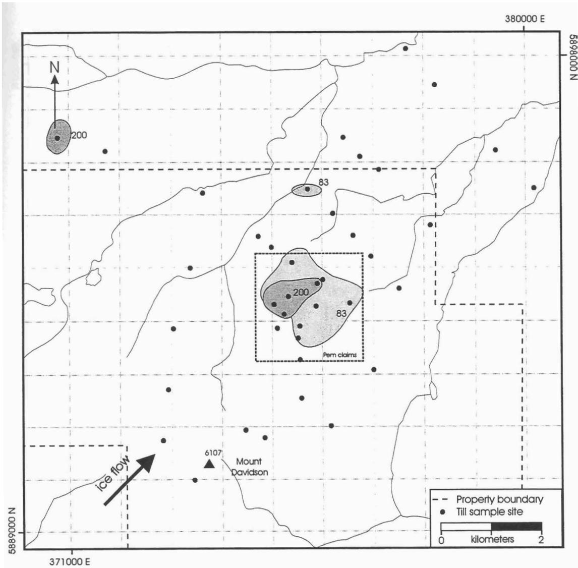
Figure 27: Till dispersal anomaly pattern for zinc (Zn), contoured at 83 and 200 ppm, Blackwater-Davidson claims.
