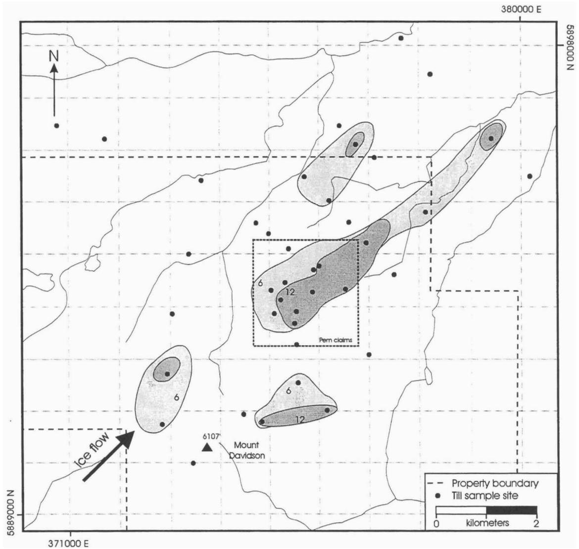
Figure 28: Till dispersal anomaly pattern for gold (Au), contoured at 6 and 12 ppb, Blackwater-Davidson claims.
