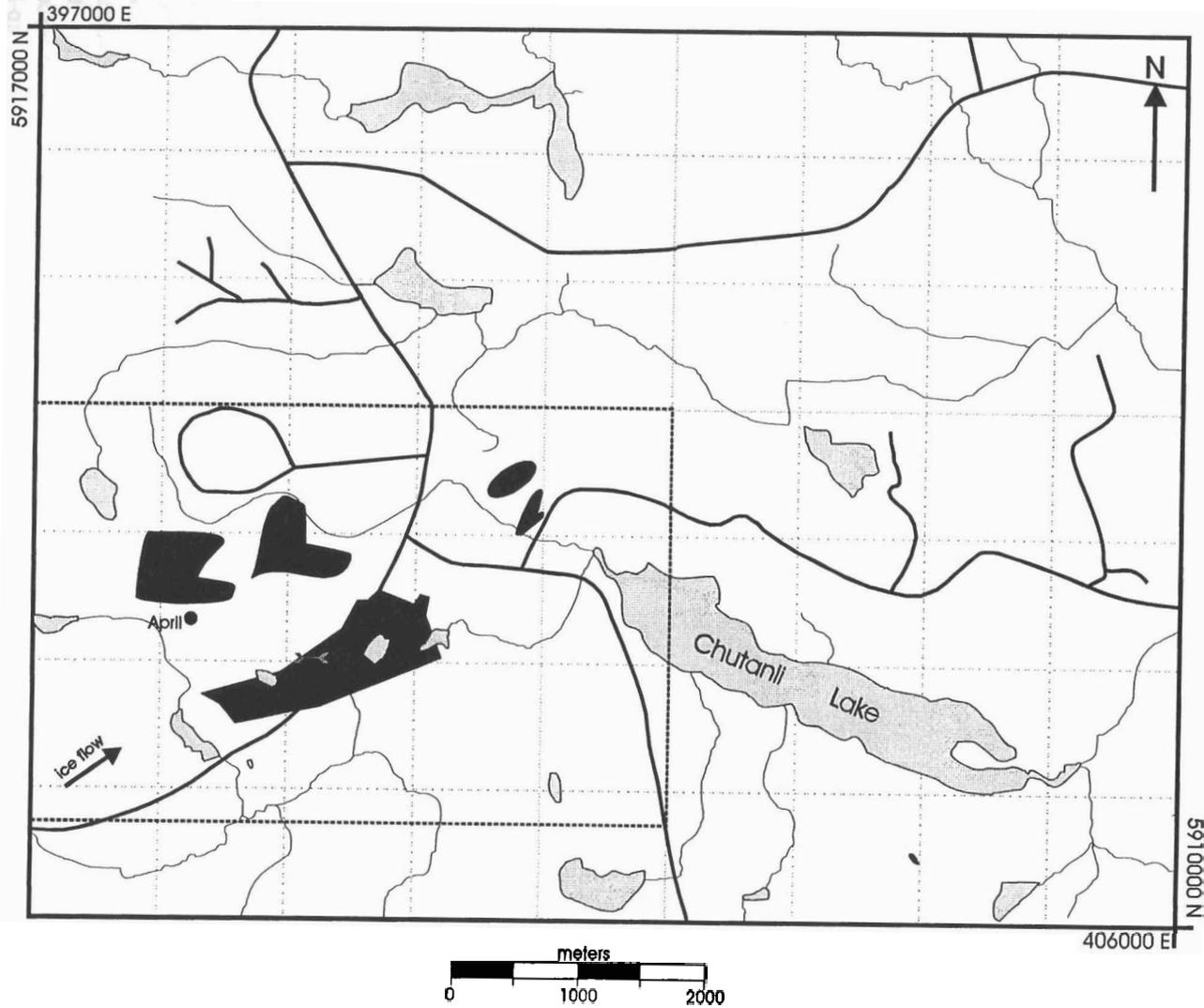
Figure 12: Soil dispersal pattern for arsenic (As) over 37 ppm, dark pattern on the CH claims (Edwards and Campbell, 1992).
