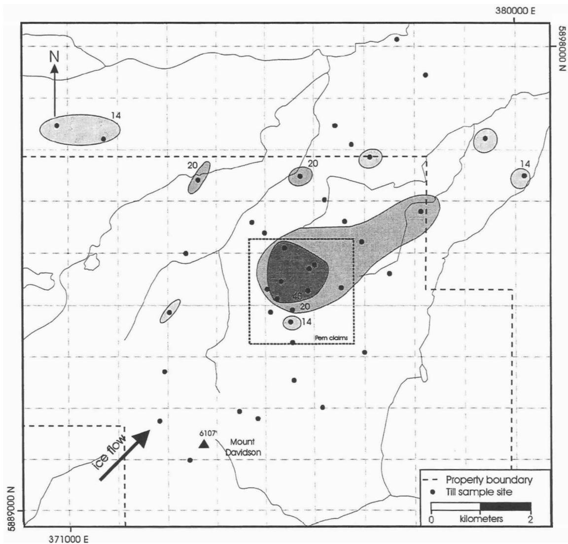
Figure 26: Till dispersal anomaly pattern for lead (Pb), contoured at 14, 20 and 40 ppm, Blackwater-Davidson claims.
